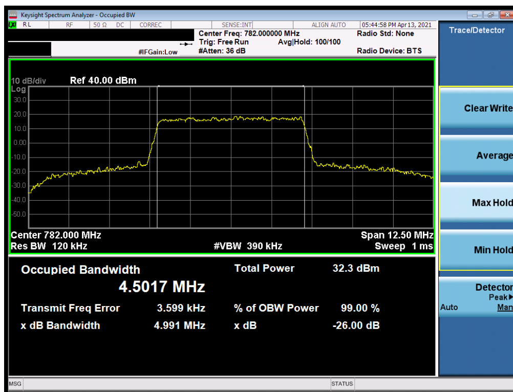
Plot 7-20. Occupied Bandwidth Plot (LTE Band 13 - 5MHz 16-QAM - Full RB)
