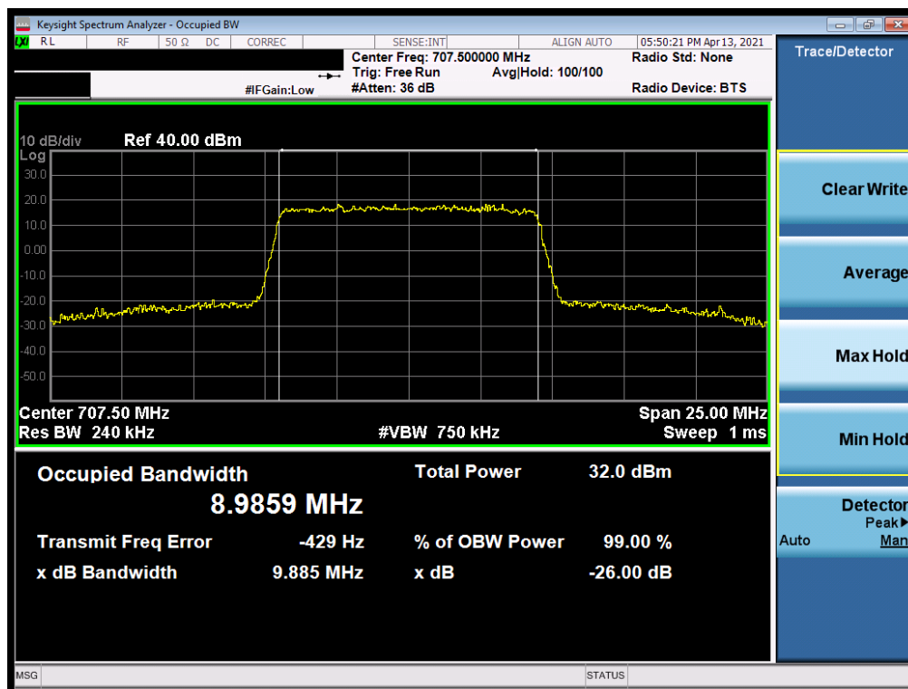
Plot 7-10. Occupied Bandwidth Plot (LTE Band 12 - 10MHz 16-QAM - Full RB)
