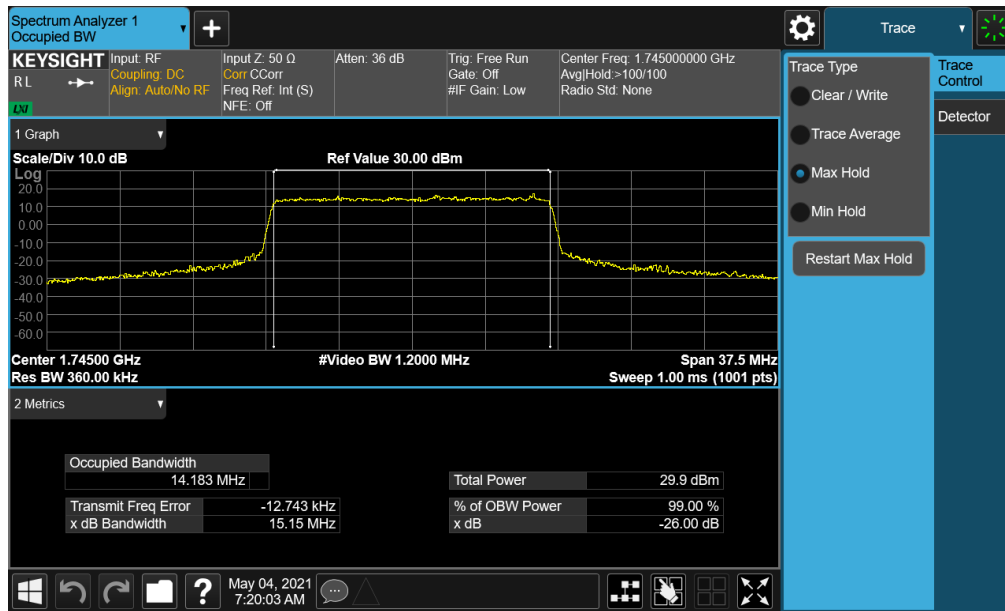
Plot 7-83. Occupied Bandwidth Plot (NR Band n66 - 15.0MHz CP-OFDM QPSK - Full RB)
