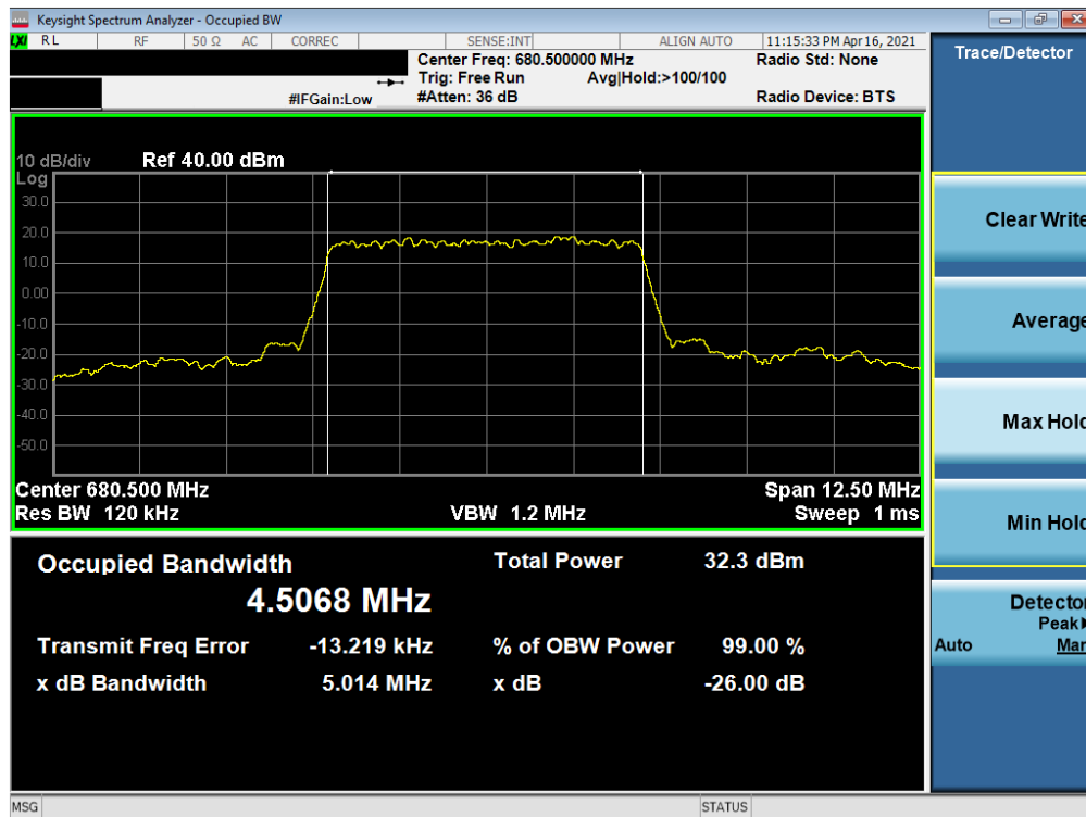
Plot 7-30. Occupied Bandwidth Plot (NR Band n71 - 5MHz DFT-s-OFDM BPSK - Full RB)
