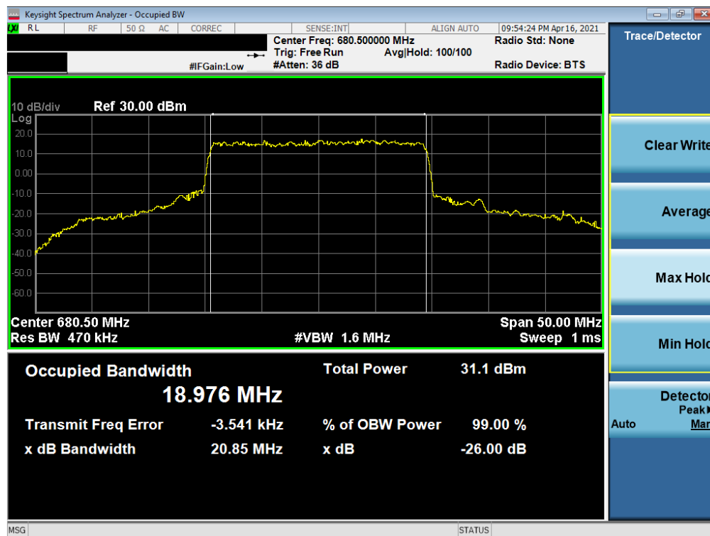
Plot 7-22. Occupied Bandwidth Plot (NR Band n71 - 20MHz CP-OFDM QPSK - Full RB)
