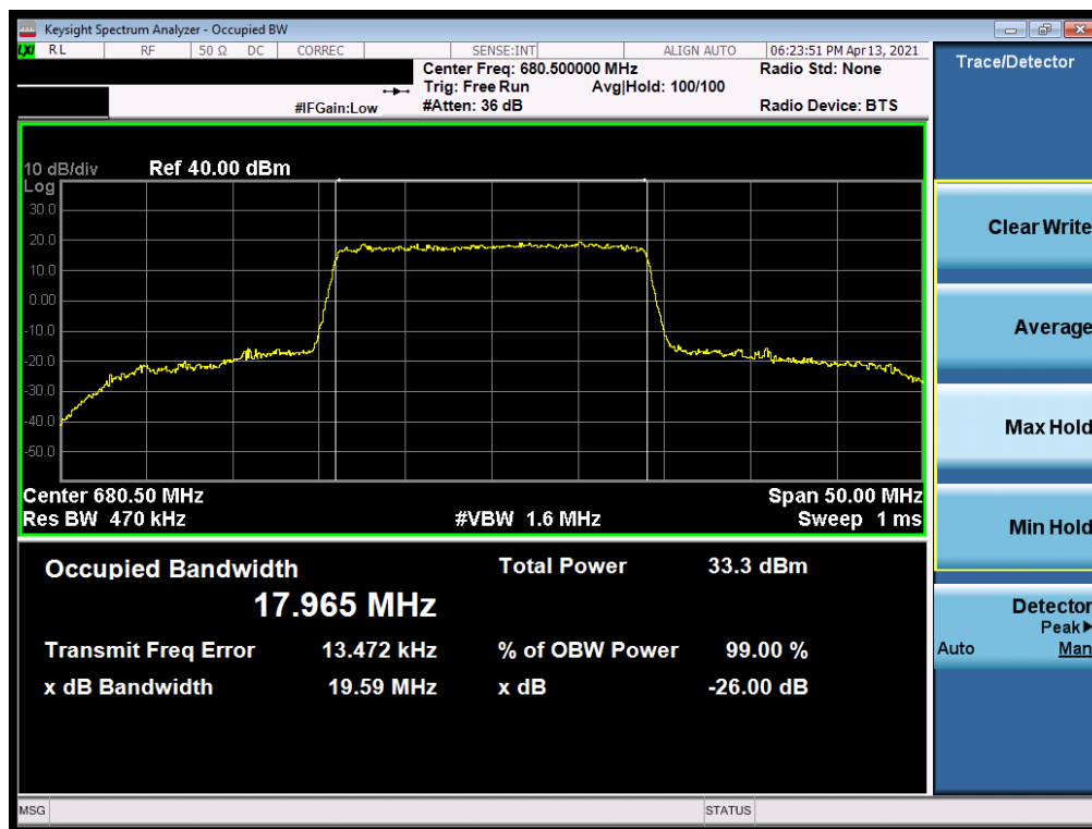
Plot 7-1. Occupied Bandwidth Plot (LTE Band 71 - 20MHz QPSK - Full RB)
