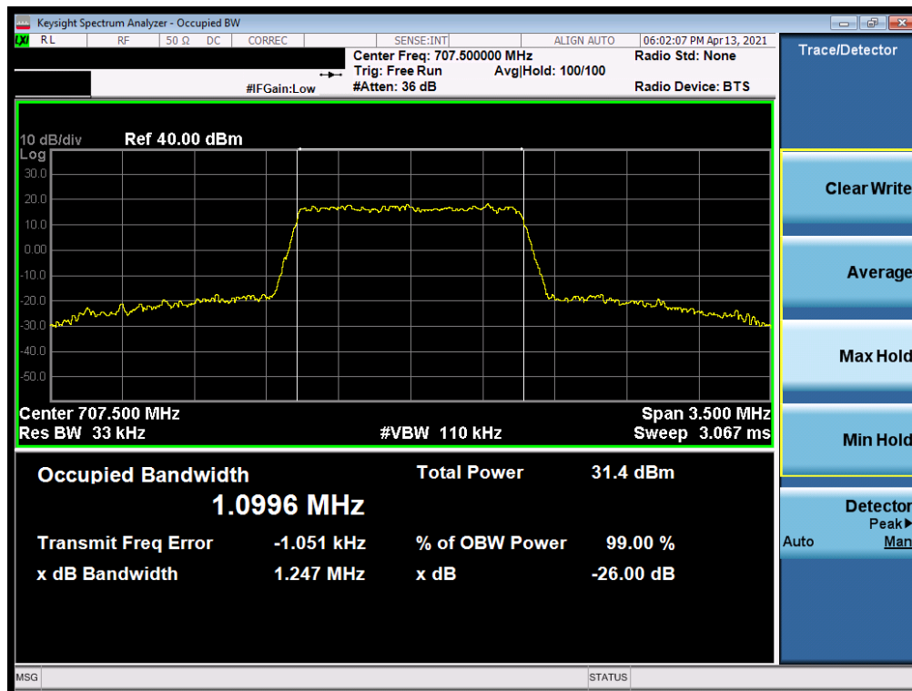
Plot 7-16. Occupied Bandwidth Plot (LTE Band 12 – 1.4MHz 16-QAM - Full RB)
