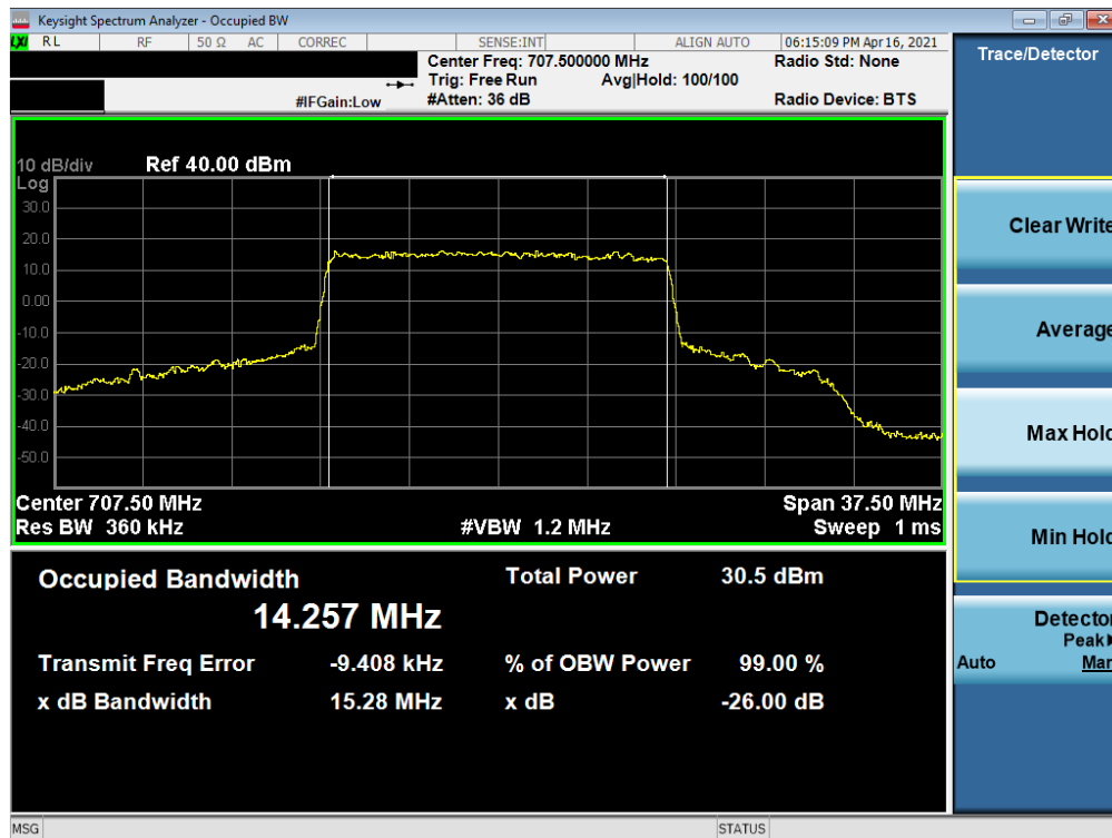
Plot 7-34. Occupied Bandwidth Plot (NR Band n12 - 15MHz CP-OFDM QPSK - Full RB)
