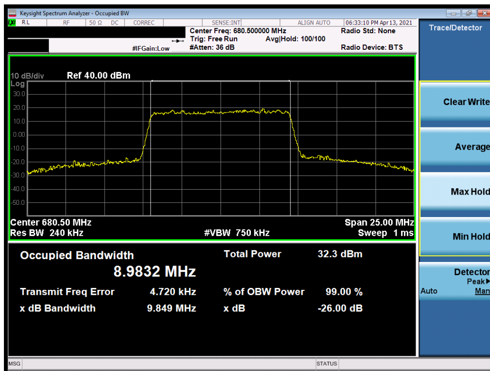
Plot 7-6. Occupied Bandwidth Plot (LTE Band 71 - 10MHz 16-QAM - Full RB)
