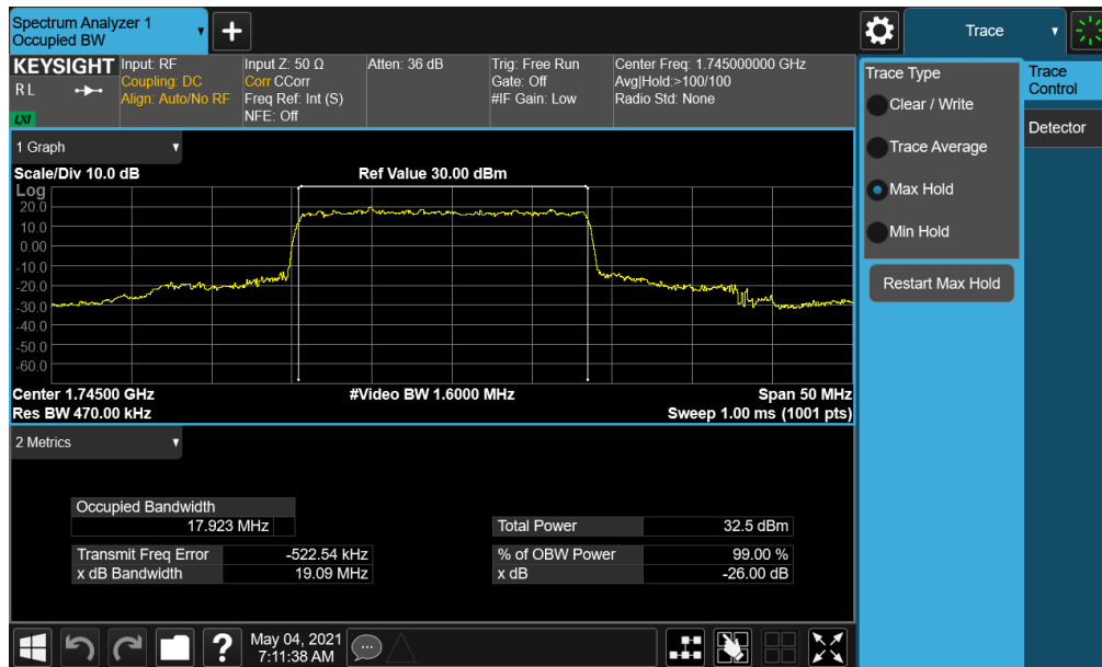
Plot 7-79. Occupied Bandwidth Plot (NR Band n66 - 20.0MHz DFT-s-OFDM BPSK - Full RB)
