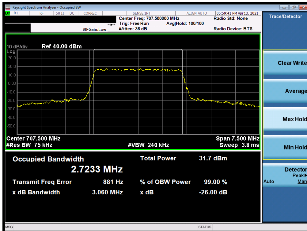
Plot 7-14. Occupied Bandwidth Plot (LTE Band 12 - 3MHz 16-QAM - Full RB)
