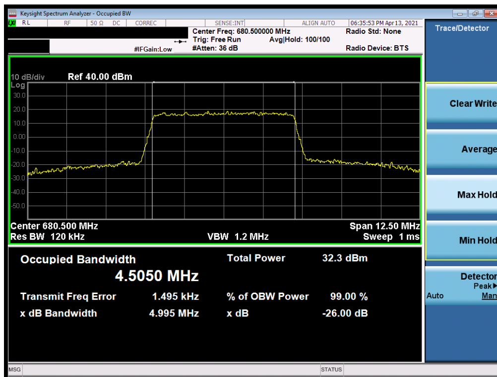
Plot 7-8. Occupied Bandwidth Plot (LTE Band 71 - 5MHz 16-QAM - Full RB)
