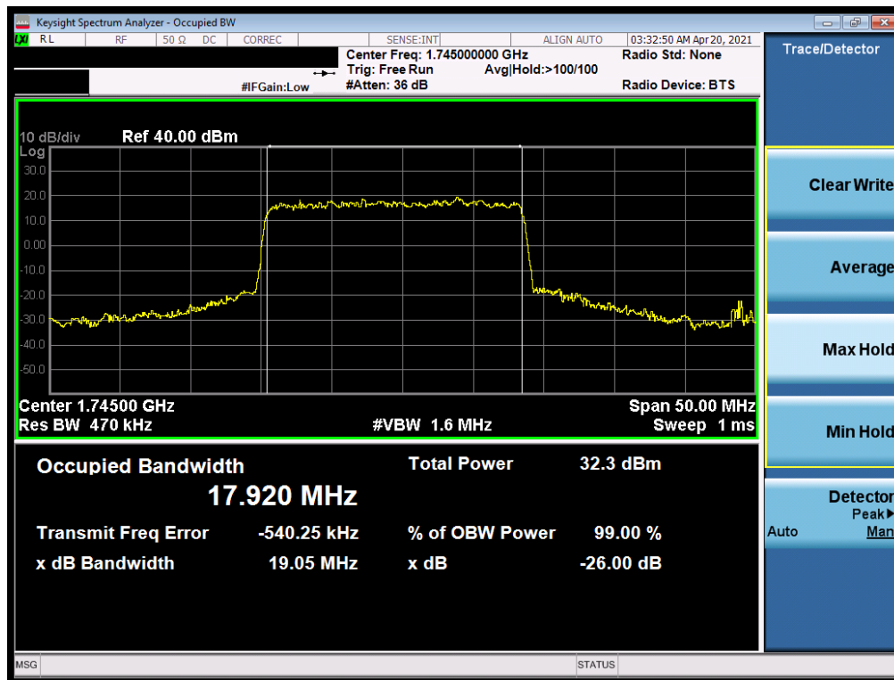
Plot 7-61. Occupied Bandwidth Plot (NR Band n66 - 20.0MHz DFT-s-OFDM BPSK - Full RB)
