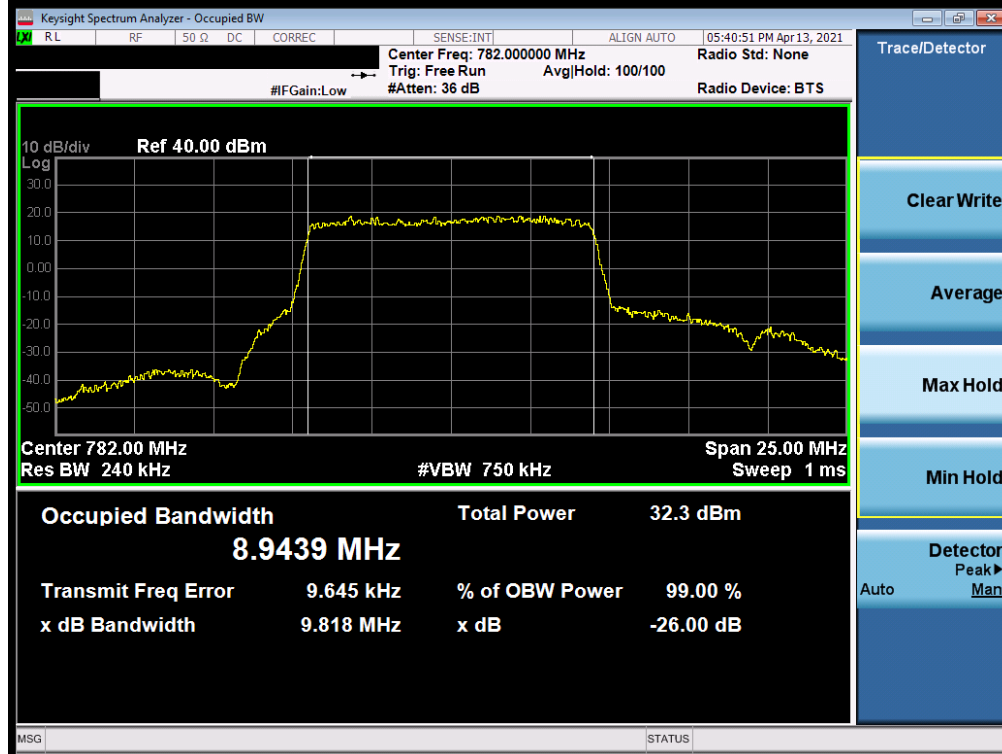
Plot 7-18. Occupied Bandwidth Plot (LTE Band 13 - 10MHz 16-QAM - Full RB)
