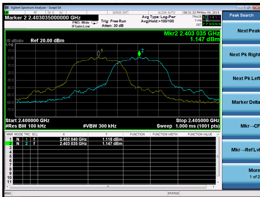
TEST PLOT FOR FREQUENCY SEPARATION
