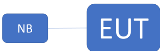
Fig. 2-2 Conducted (Antenna Port) Emission Configuration
