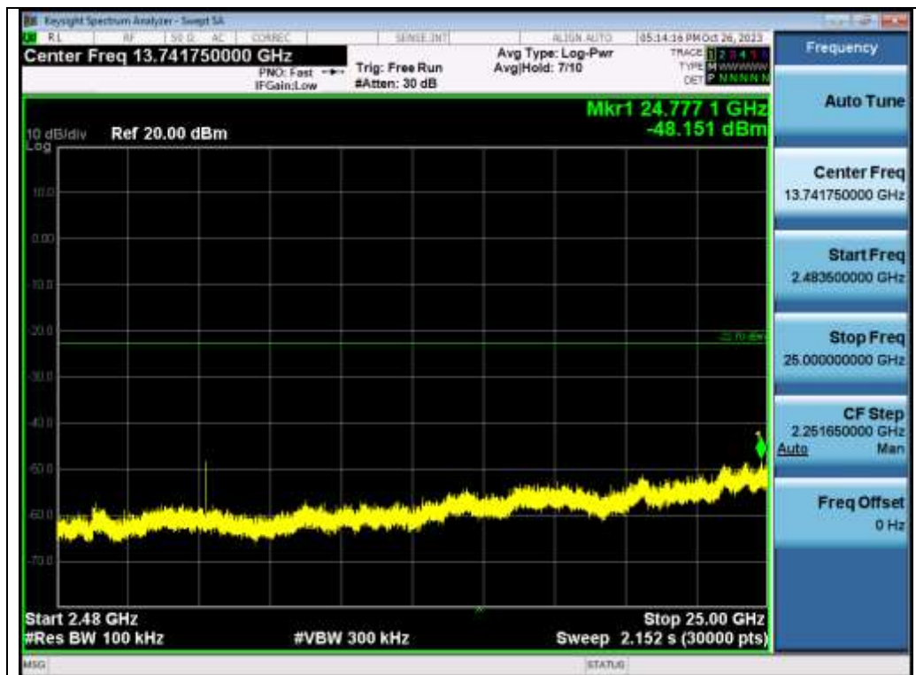
Test_Graph_LE1M_ANT1_2402_1Mbps_Higher Band Emissions
