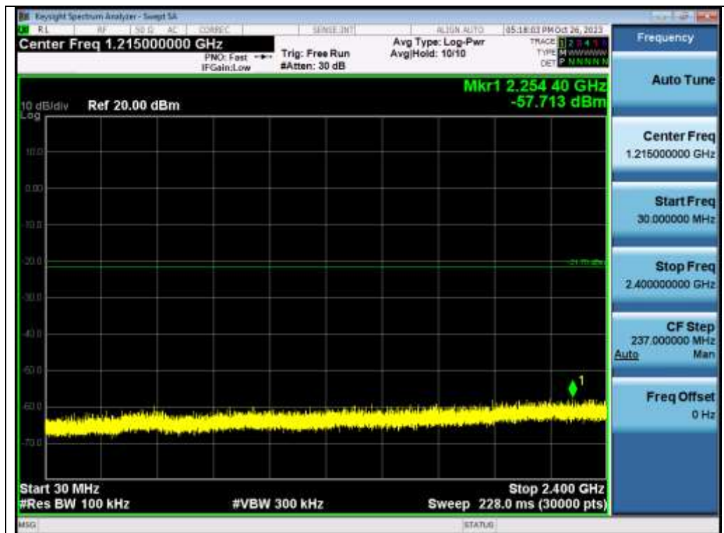
Test_Graph_LE1M_ANT1_2440_1Mbps_Lower Band Emissions
