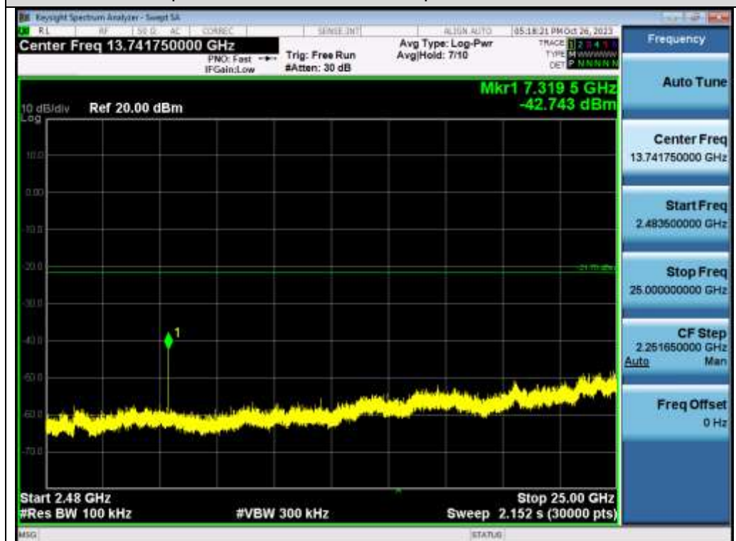
Test_Graph_LE1M_ANT1_2440_1Mbps_Higher Band Emissions
