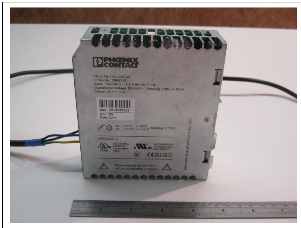
Photograph A3-7: Power supply TRIO-PS/1AC/24DC/5
