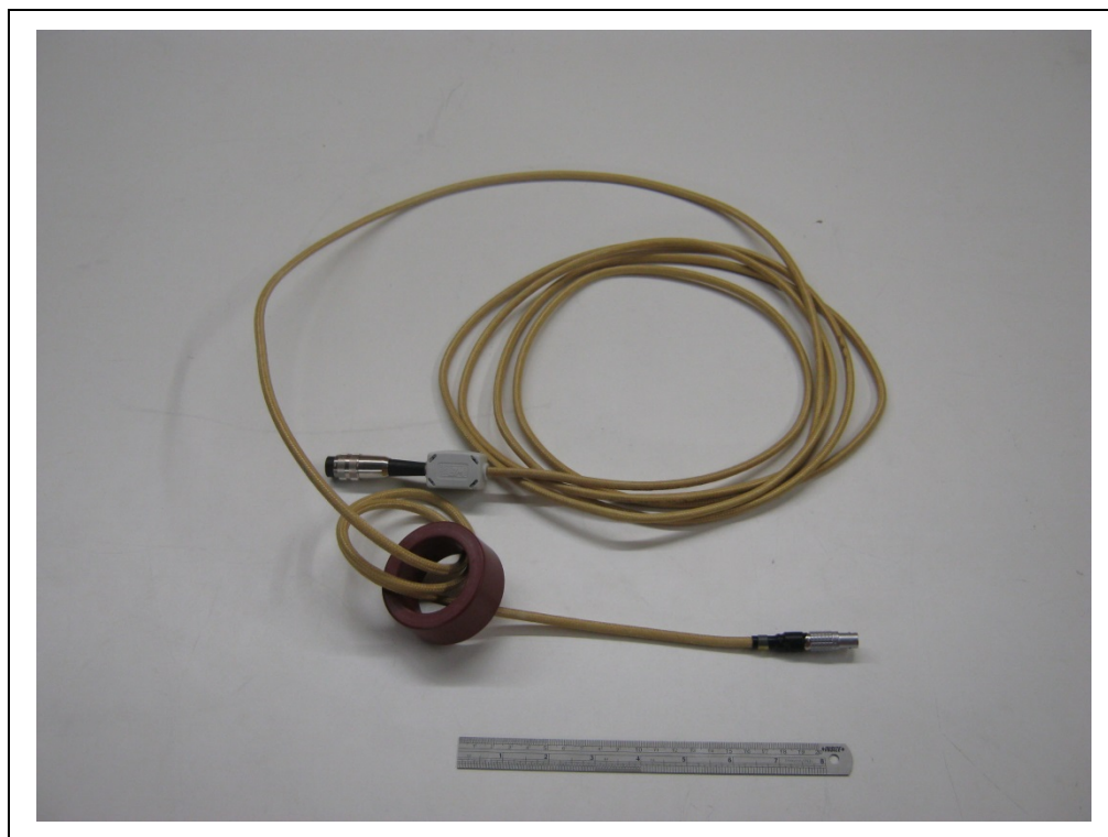
Photograph A3-4: Connection cable Axon control unit to stator unit with ferrites
