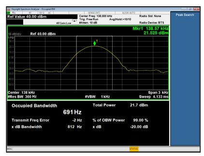
Note: The measured signal is Cw-ike, adjusting the RBW per C63.10 would not be practical since measurement bandwidth will always follow the RBW. The RBW is set to 300 Hz to perform the occupied bandwidth test.
