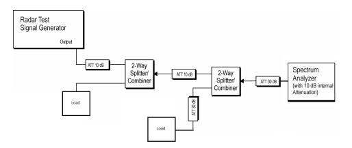
Waveform Calibration Test Setup Diagram
