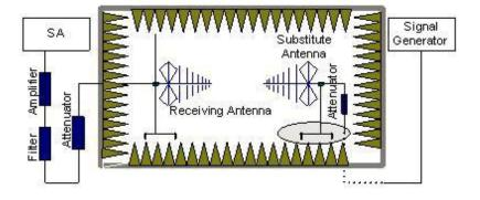
In the chamber, an substitution antenna for the frequency band of interest is placed at the reference point of the chamber. An RF Signal source for the frequency band of interest is connected to the substitution antenna with a cable that has been constructed to not interfere with the radiation pattern of the antenna. A power  $(P_{\text{Mea}})$  is applied to the input of the substitution antenna, and adjust the level of the signal generator output until the value of the
