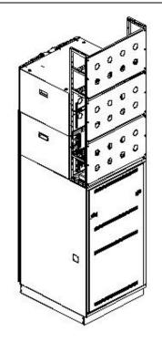
Fig. 4.2-18 Feeder Fixing Rack after Installation
