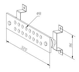
Fig. 6.2-1 Appearance of the Grounding Copper Bar
