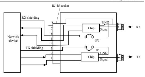
Fig. 8.3-2 Wiring of the Impedance Converter
