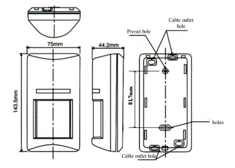
Fig. 9.2-4 Structure of Infrared Sensor
