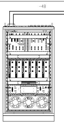
Fig. 5.3-1 RFS Power Cabling
