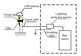
Fig. 11.2-1 Composition of the GPS Antenna Feeder System
