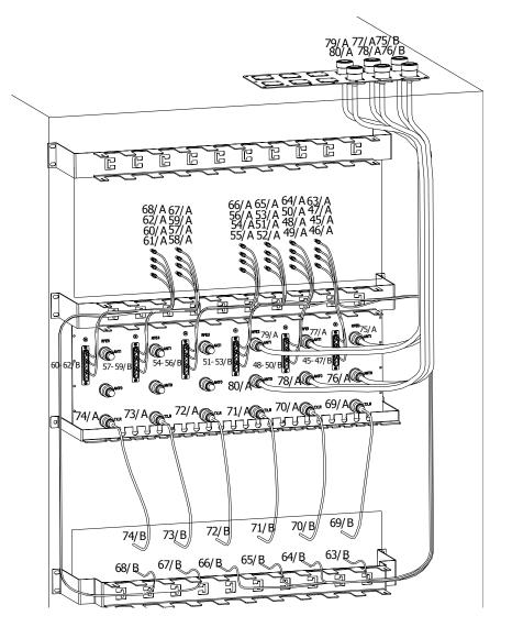
Fig. 7.3-6 RF Cabling in the RFS
