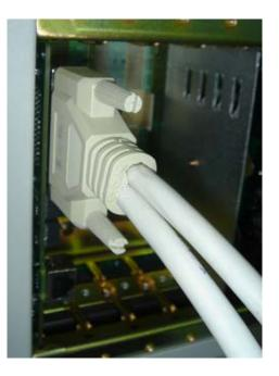
Fig. 8.1-1 D\_SUB44-core Connector Connecting BDS
