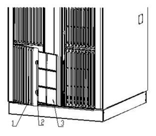
1. Plastic decoration panel 2. Pin 3. Dust-filtering network board
