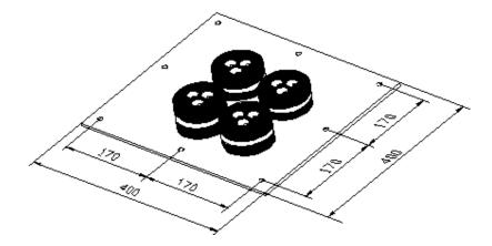
Fig. 10.4-4 Structure of the Feeder Window
