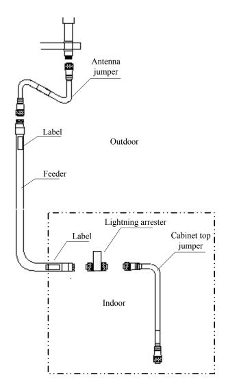
Fig. 10.4-5 Structure of a BTSB Feeder
