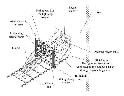
Fig. 6.2-4 Installing the Lightning Arrester Frame
