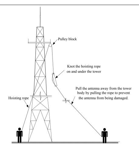
Fig. 10.4-1 Hoisting an Antenna
