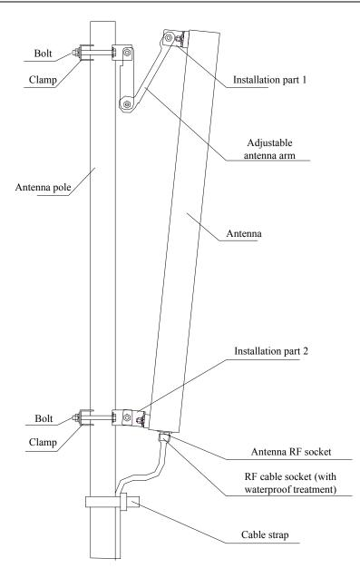
Fig. 13.15-1 Antenna Installation Checking the Feeder SWR
