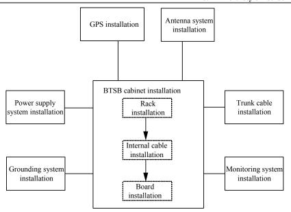
Fig. 1.1-3 BTSB Installation Hardware
