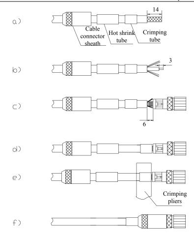
Fig. 8.2-3 Assembling DDF Coaxial Cable Plug
