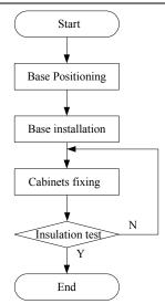
Fig. 4.2-10 Base Installation Flow
