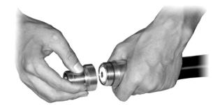
Fig. 10.4-10 Connecting the Front Part and the Back Part of the Feeder Connector
