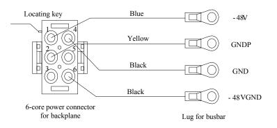
Fig. 5.3-3 Connection between Busbar and Backplane
