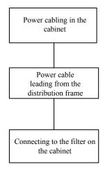
Fig. 5.2-1 Installation Flow of RFS Power
