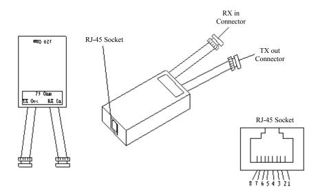
Fig. 8.3-1 Appearance and Wiring of an Impedance Converter
