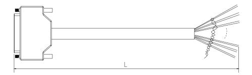
Fig. 8.1-3 Structure of 120  $\Omega$  E1 Cable
