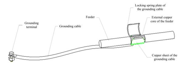
Fig. 6.2-2 Structure of the Grounding Clip
