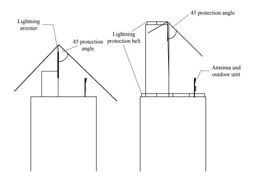
For details of the lightning protection to the antenna, see Fig. 10.5-1.
