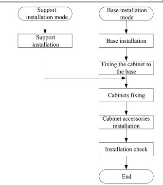
Fig. 4.2-1 Cabinet Installation Flow
