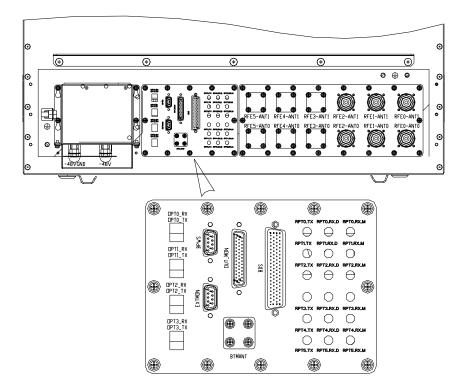
The layout of the interface board on the top of RFS cabinet is shown in Fig. 7.3-3.
