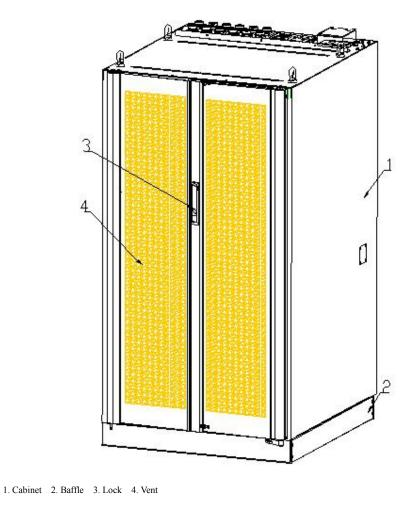
Fig. 4.2-8 Cabinet after Installation
