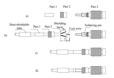
Fig. 8.2-1 Assembly of the CC4Y-J32 Coaxial Cable Connector
