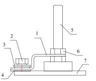
1. Pressure plate 2.  $M10 \times 25$  bolts 3 Washer 4. Insulation pad 5. Cabinet support 6. Retaining nut 7. Base
