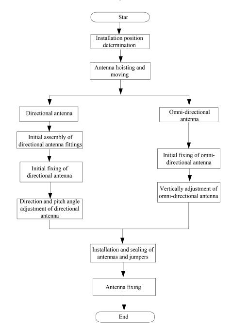
Fig. 10.3-1 Antenna Installation Flow
