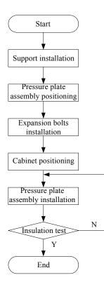
Fig. 4.2-3 Support Installation Flow
