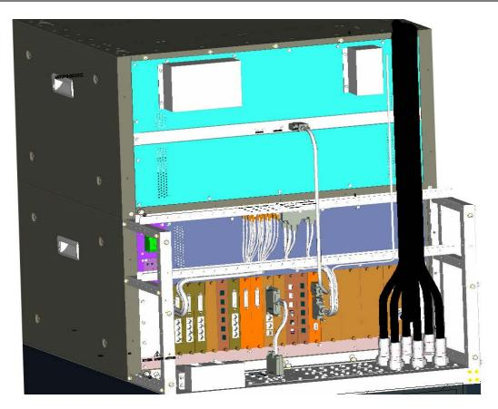
Fig. 7.3-5 RF Cable Interface in RFS
