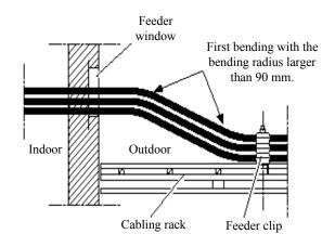
Fig. 10.4-14 Introducing Feeders into the Equipment Room (Method 1)
