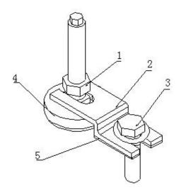
1. Locking nut 2. Pressure plate 3. M10X25 bolt 4. Support 5. Insulating washer
