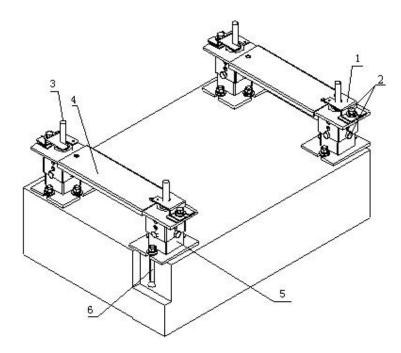
1. Pressure plate 2. M10  $\times$  25 bolts 3 Cabinet support 4. Bracket 5. Base 6. M10  $\times$  40 embedded expansion (12  $\phi$  bit, 43 hole depth)
