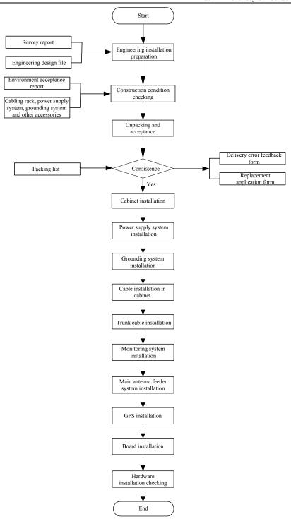
Fig. 1.2-1 Hardware Installation Flow
