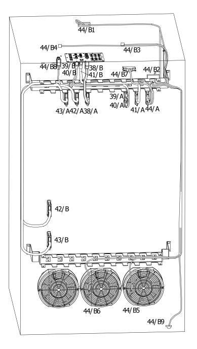
Fig. 7.3-4 Signal and Monitoring Cabling in the RFS
