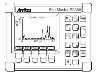
Fig. B.6-1 Antenna Feeder DTF Measurement
