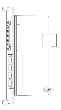
Fig. 12.4-2 Structure of a Back Interface Board
