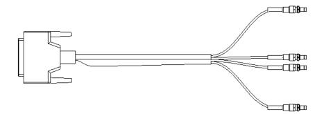
Fig. 8.1-2 Structure of 75  $\Omega$  E1 Cable
