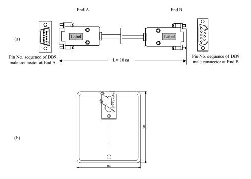
Fig. 9.2-2 Installation of Temperature-Humidity Converter
