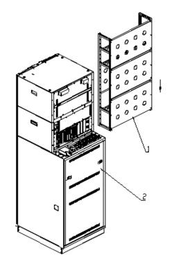
1. Feeder fixing rack 2. RFS cabinet
