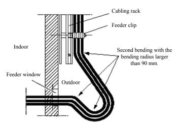
Fig. 10.4-15 Introducing Feeders into the Equipment Room (Method 2)
