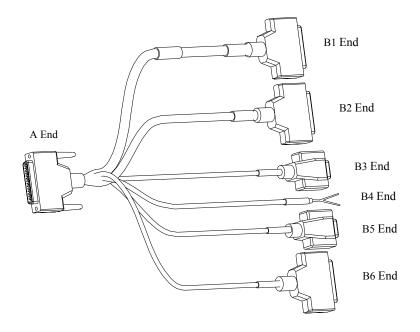
Fig. 9.1-1 Structure of External Monitoring Cable of RFS
