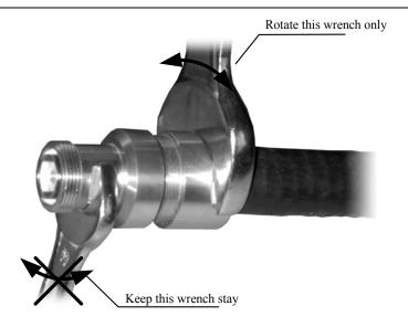
Fig. 10.4-11 Fixing the Front Part and the Back Part of the Feeder
