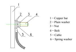
Fig. 5.3-4 Connecting Power Cable (1)
