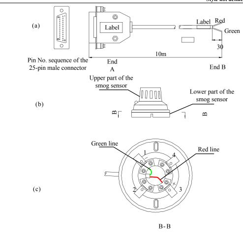
Fig. 9.2-1 Installing the Smog Sensor Base
