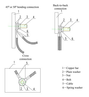
Fig. 5.3-5 Connecting Power Cable (2)
