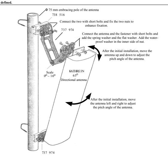
Fig. 10.4-2 Installing the KATHRAIN Antenna
