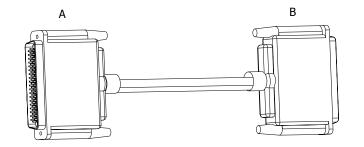
Fig. 7.4-1 Interconnection Cables between BDS and RFS Cabinets
