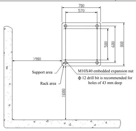
Fig. 4.2-6 Positions of Installation Holes of Cabinet Supports
