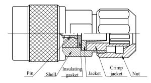
Fig. 11.4-3 Structure of the N-J7A Cable Connection Part
