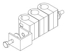
Fig. 10.4-13 Three-feeder Clip
