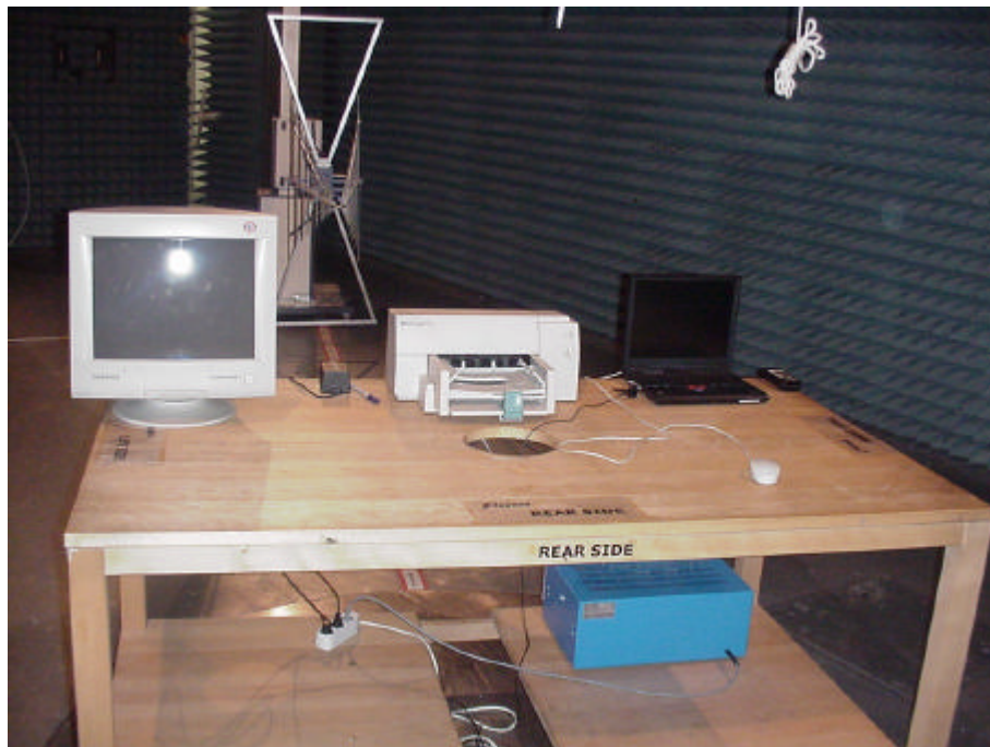
Picture 2 : Setup for radiated emission measurement (front view)
