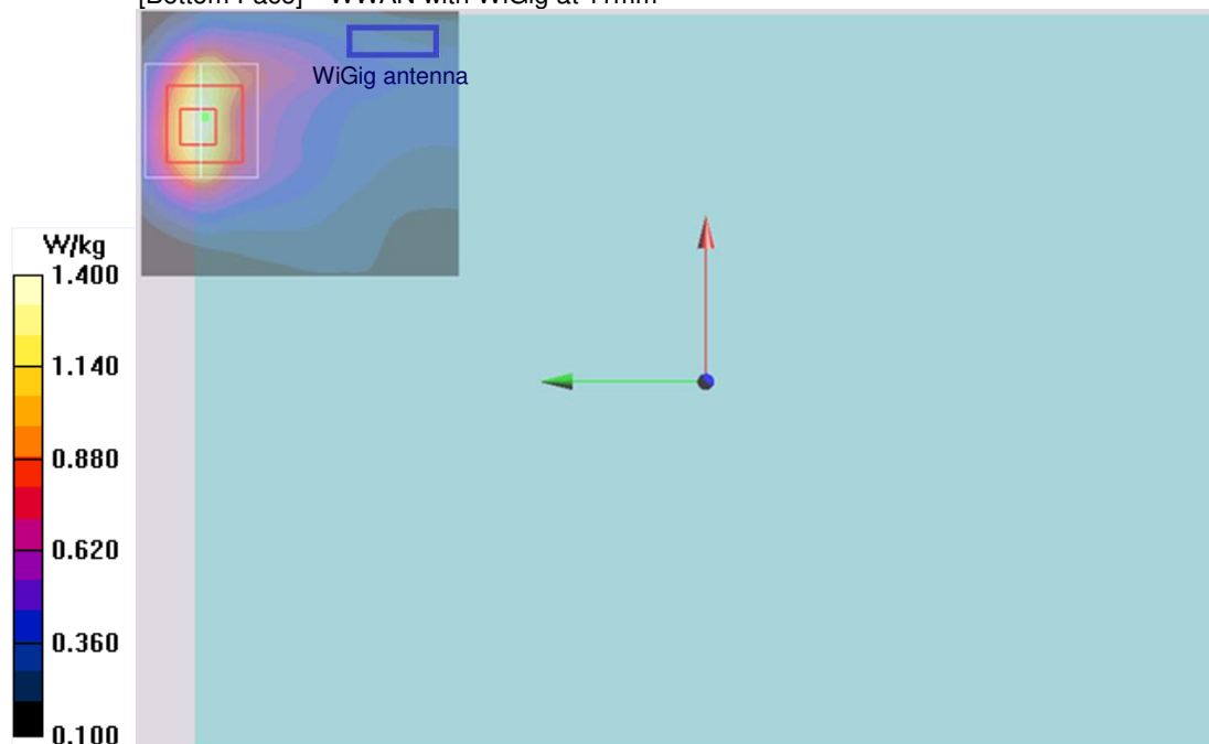
[Bottom Face] WWAN with WiGig at 11mm
