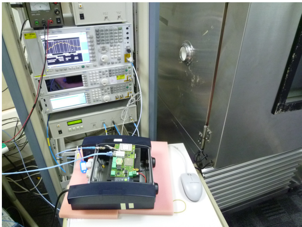
Photograph 4: Set-up for Conducted testing
