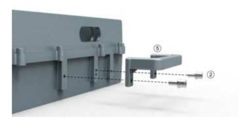
2. Attach and fasten the Bracket I to the back of HPRU with screws M6×14 using T5 Wrench.
