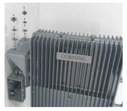
7. Fasten the Bracket I and II with screws M6×14.
