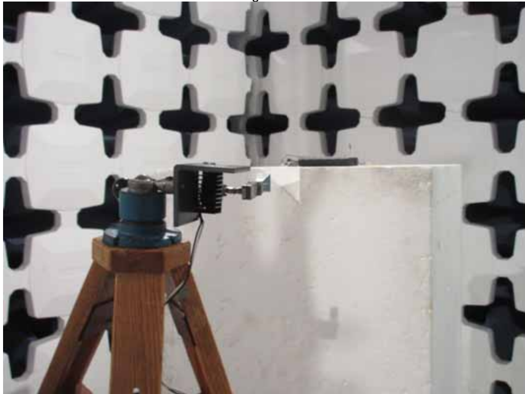
Test Setup for Radiated Emissions – 26.5GHz to 40GHz, Horizontal Polarization
