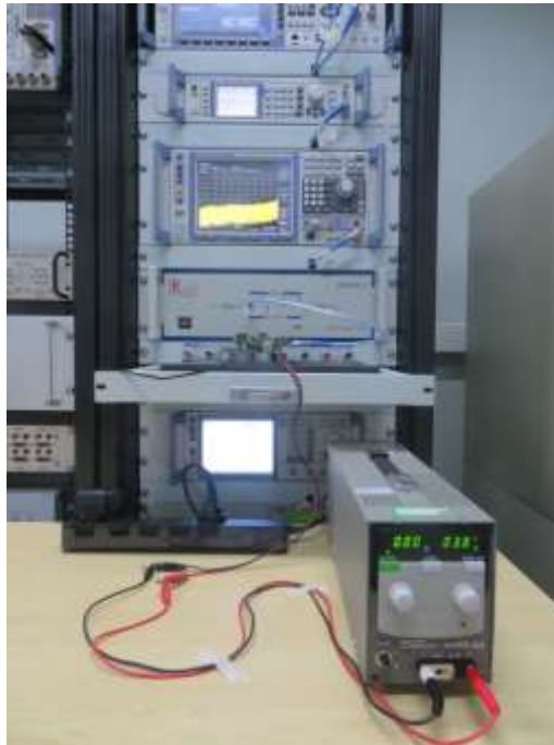
Photograph 1: Set-up for RF Output Power Measurement
