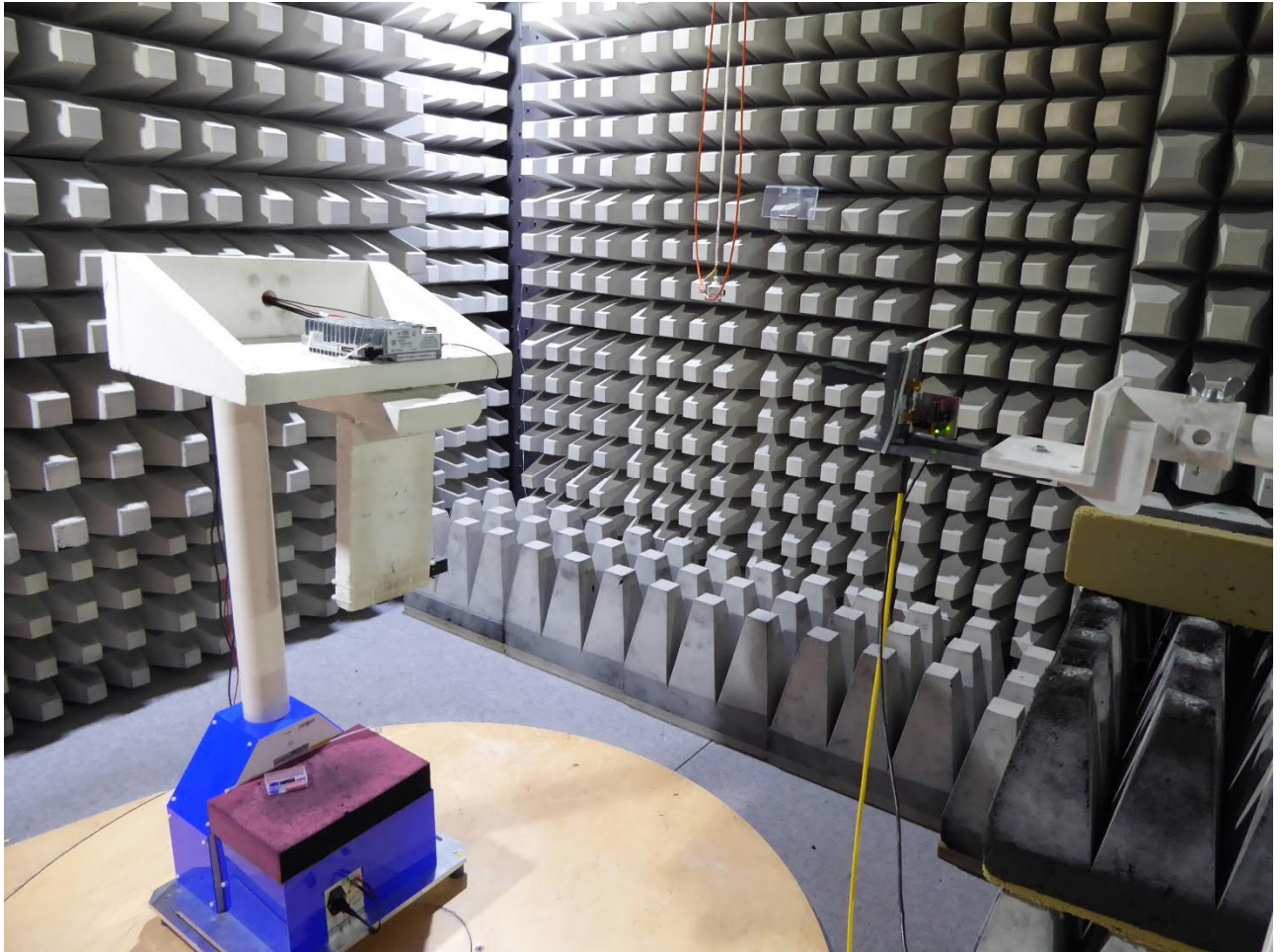
Test setup fully anechoic chamber (26.5 - 40 GHz)
