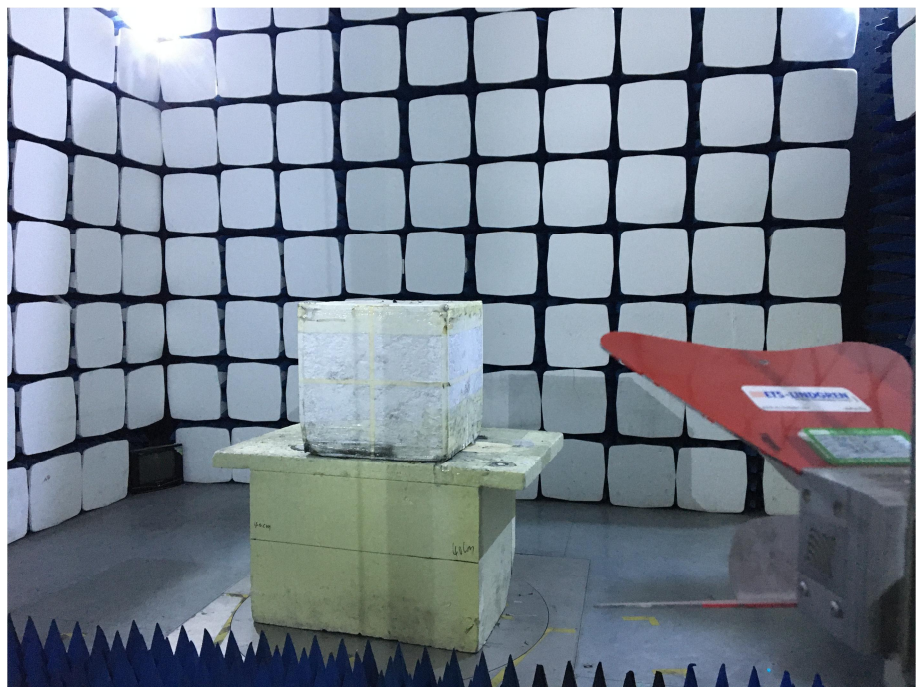
Radiation Emission Test Setup (1GHz to 18GHz)
