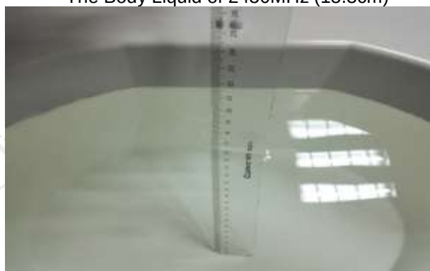
The Body Liquid of 5000-6000MHz (16.5cm)
