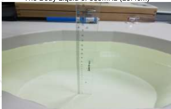
The Body Liquid of 1900MHz (16.4 cm)
