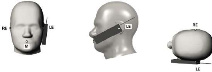
Positioning for Ear / 15° Tilt
