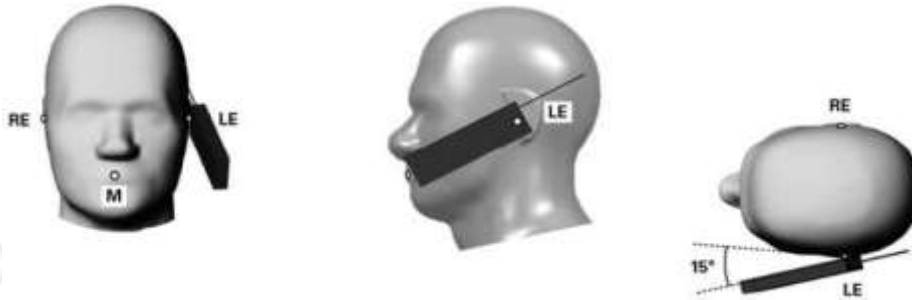
Positioning for Ear / 15° Tilt
