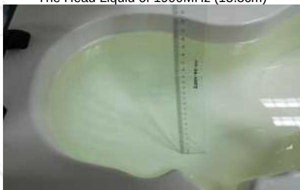
The Head Liquid of 835MHz (15.3cm)
