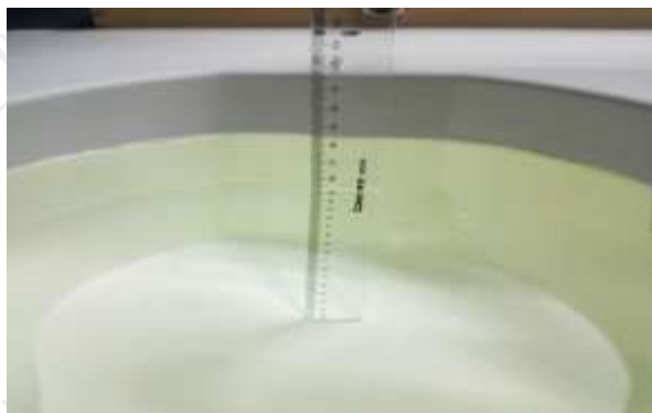
The Body Liquid of 1800MHz (15.2 cm)
