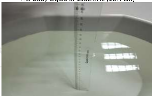
The Body Liquid of 2600MHz (16.5cm)
