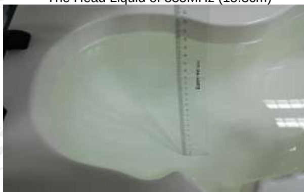
The Head Liquid of 2600MHz (15.1cm)
