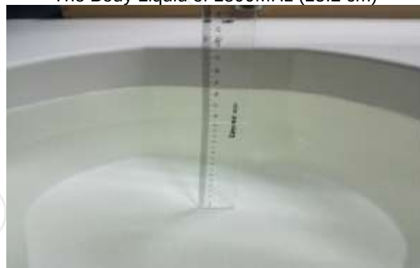
The Body Liquid of 2450MHz (15.3cm)
