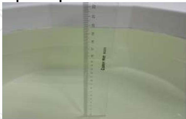
The Body Liquid of 835MHz (15.4cm)
