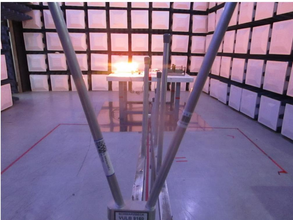
**Radiated Emissions Test Photos****Above 1 GHz**
