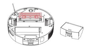
Remove the Anti-Tangle Rubber Brush, pull out the bearings at both ends, and clean any hair or dirt wrapped around the brush. You can use the provided small cleaning tool for this.
