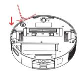
When you hear a clicking sound, it means the Side Brush has been properly installed.
