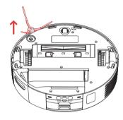
Clean the Side Brush and its mounting shaft, then reinstall it.
