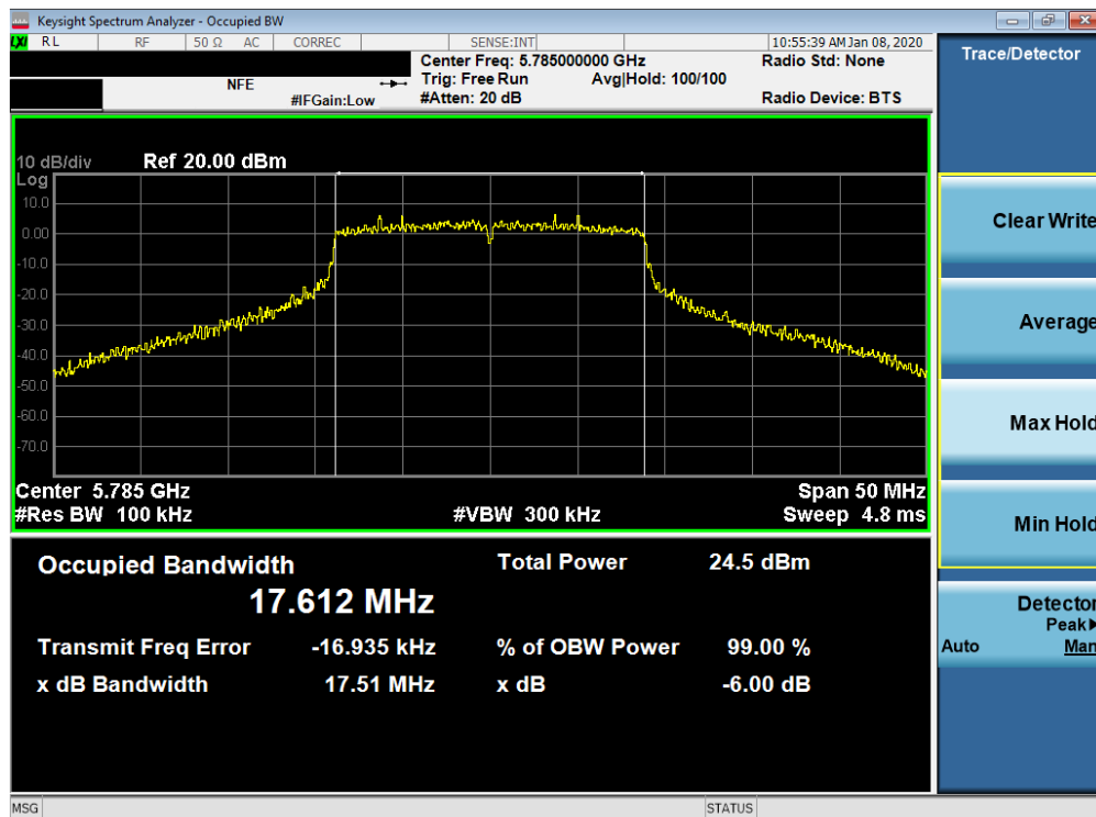
Plot 7-118. 6dB Bandwidth Plot SISO ANT2 (20MHz BW 802.11n (UNII Band 3) – Ch. 157)
