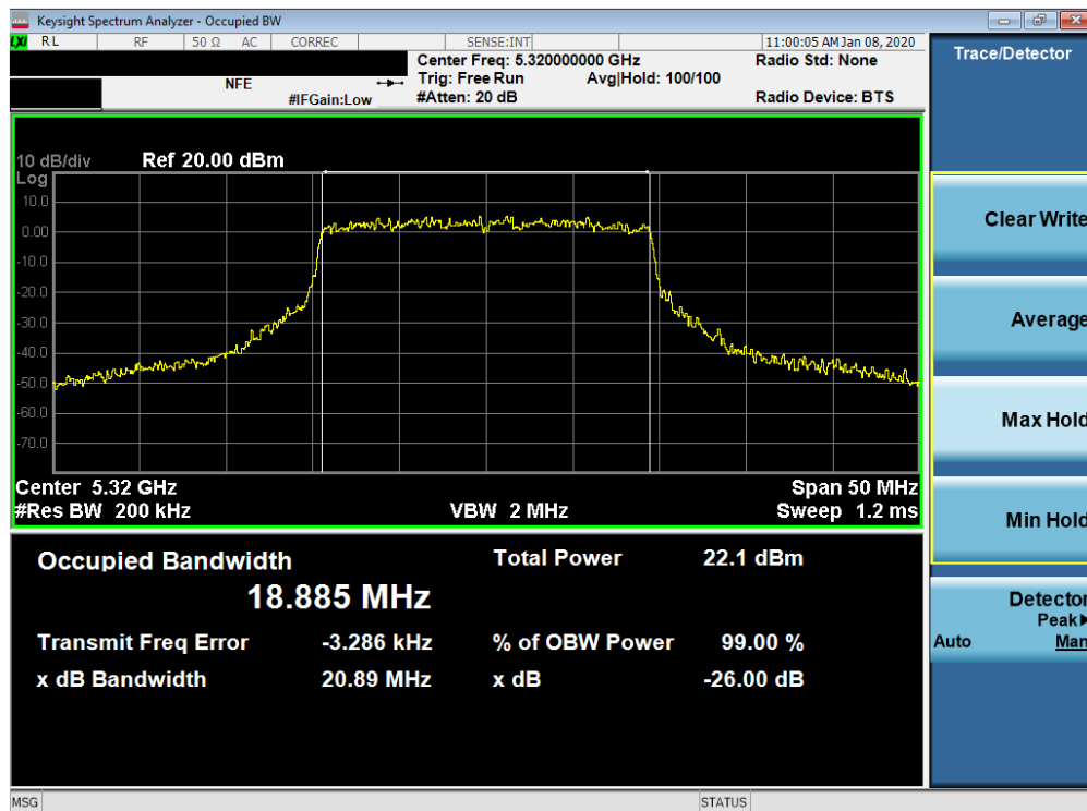
Plot 7-73. 26dB Bandwidth Plot SISO ANT2 (20MHz BW 802.11ax (UNII Band 2A) – Ch. 64)
