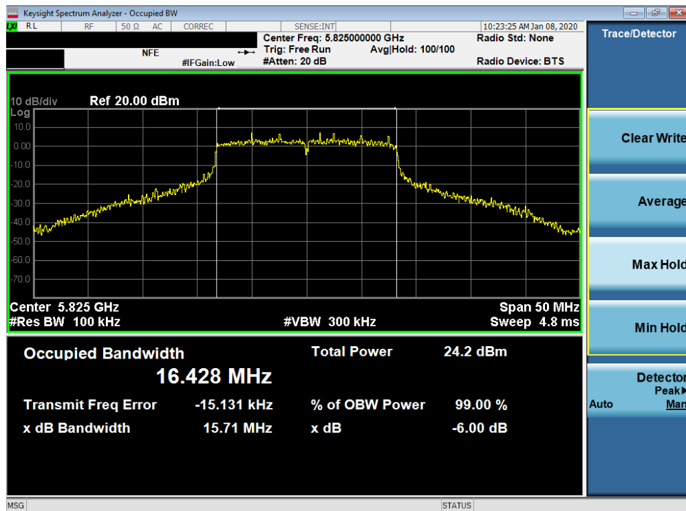
Plot 7-116. 6dB Bandwidth Plot SISO ANT2 (802.11a (UNII Band 3) – Ch. 165)
