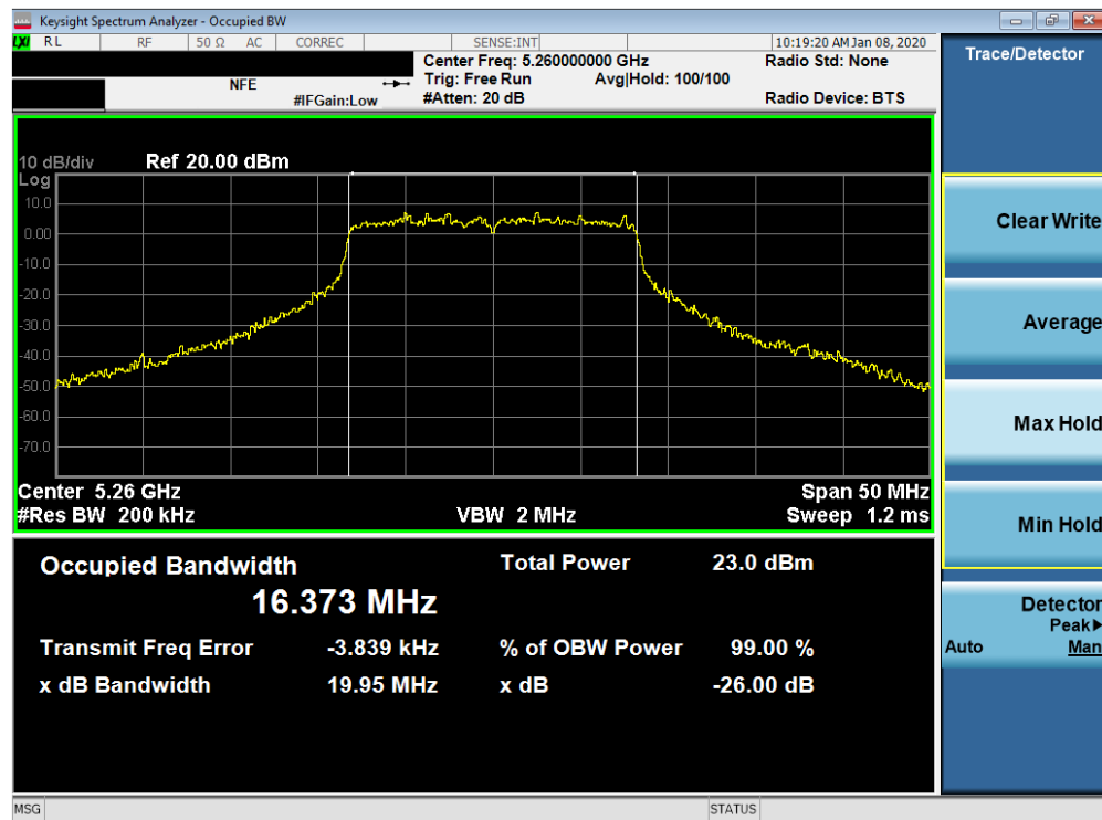
Plot 7-65. 26dB Bandwidth Plot SISO ANT2 (802.11a (UNII Band 2A) – Ch. 52)
