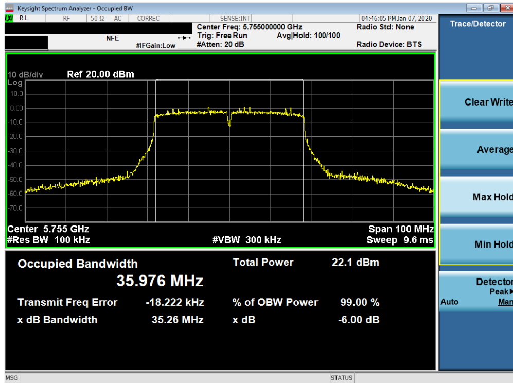
Plot 7-108. 6dB Bandwidth Plot SISO ANT1 (40MHz BW 802.11n (UNII Band 3) – Ch. 151)
