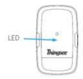
Sensor is switched on with the magnet switch tool by holding it against the sensor's magnetic switch.
