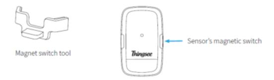
Hold the magnet switch tool against the sensor (see the pic) until the LED indicator starts to blink brightly for one minute.
