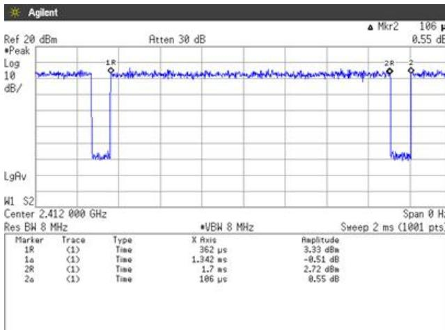
$$\text{Duty Cycle} = \frac{\text{Ton}}{(\text{Ton} + \text{Toff})} = \frac{1342[\mu\text{s}]}{(1342[\mu\text{s}] + 106[\mu\text{s}])} = 92.68[\%]$$
