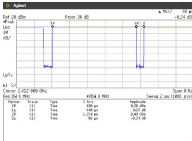
$$\text{Duty Cycle} = \frac{\text{Ton}}{(\text{Ton} + \text{Toff})} = \frac{940[\mu\text{s}]}{(940[\mu\text{s}] + 86[\mu\text{s}])} = 91.62[\%]$$
