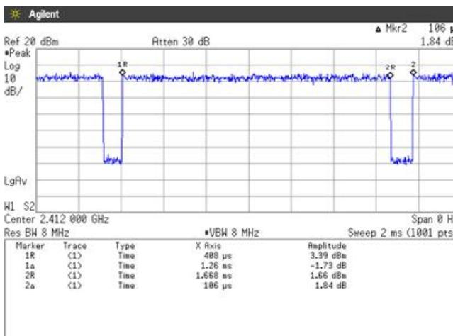
$$\text{Duty Cycle} = \frac{\text{Ton}}{(\text{Ton} + \text{Toff})} = \frac{1260[\mu\text{s}]}{(1260[\mu\text{s}] + 106[\mu\text{s}])} = 92.24[\%]$$
