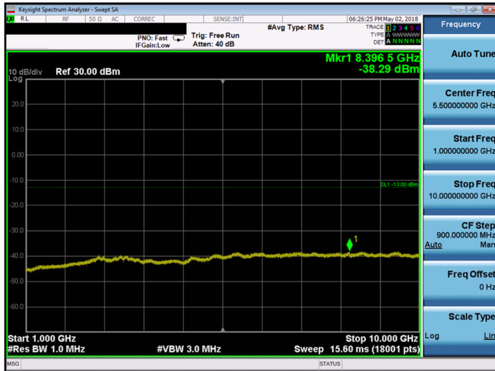
Plot 7-36. Conducted Spurious Plot (Cellular CDMA Mode - High Channel)
