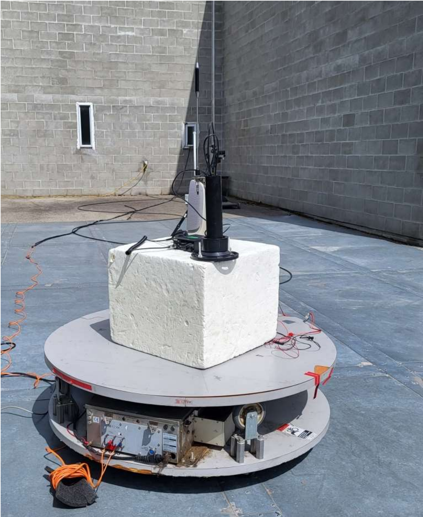
Figure E18.5 – Setup, Radiated Emissions Below 30MHz, with Accessories
