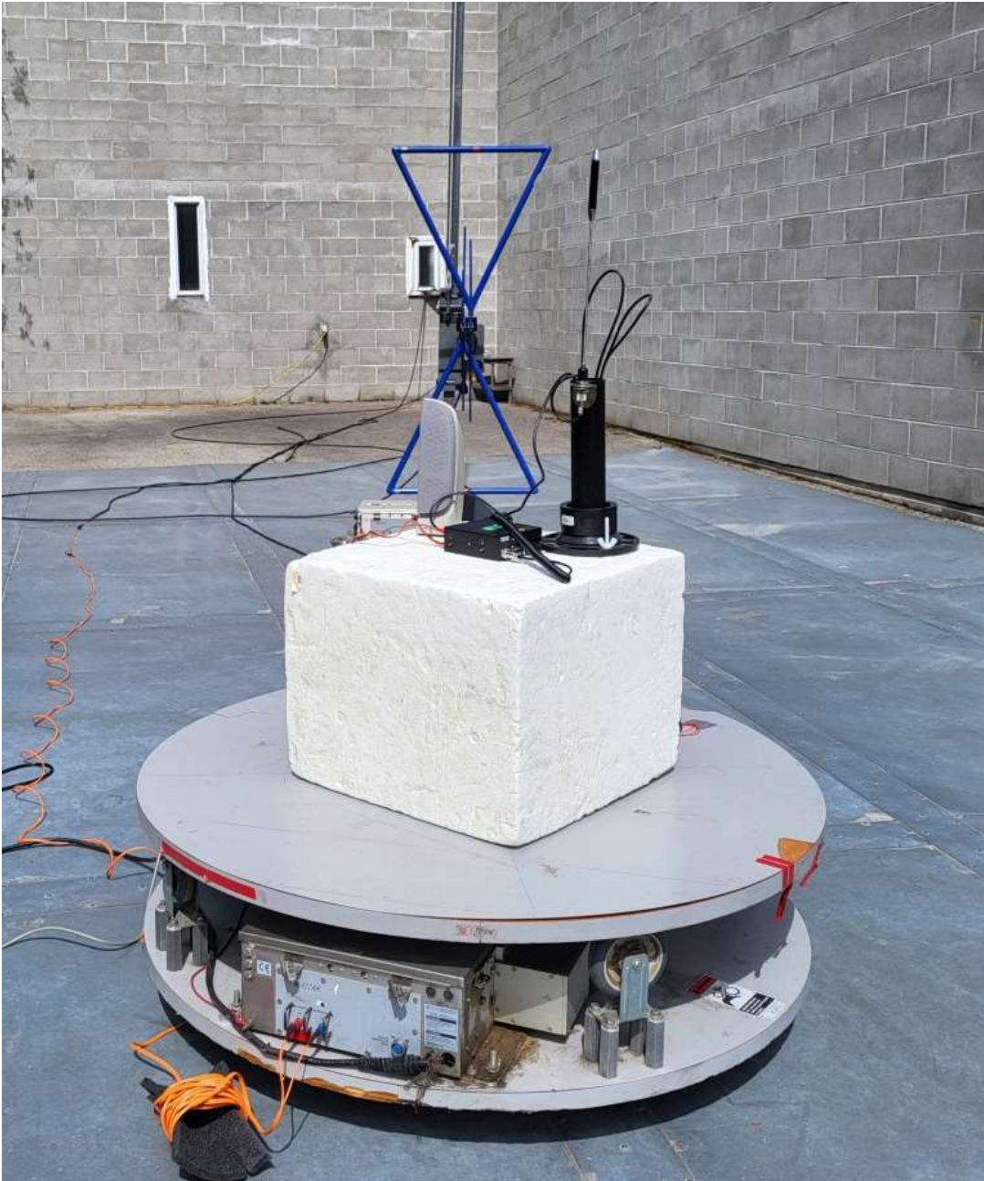
Figure E18.8 – Setup, Radiated Emissions 30 - 1000MHz, with Accessories
