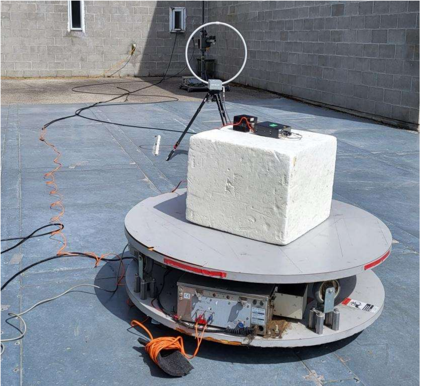
Figure E18.4 – Setup, Radiated Emissions Below 30MHz, without Accessories
