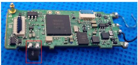
The antenna is integrated on the main PCB and no consideration of replacement. The best case gain of the antenna is 4dBi.
