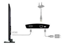
There will be an HDMI cable and USB adapter inside of the box, use the 5V-1A DC adapter to power up EZCast LAN box, and plug HDMI cable into HDMI port. We also suggest connect RJ045 port with your router to simplify setup procedures and get stable connection.
