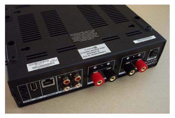
Turn the unit upside down and place the labels on the bottom of the chassis toward the rear panel. Orient all labels such that they are readable (right-side up) when looking at the rear panel as shown above.
