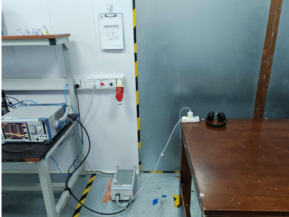
Conducted emissions at AC power line (150kHz-30MHz)
