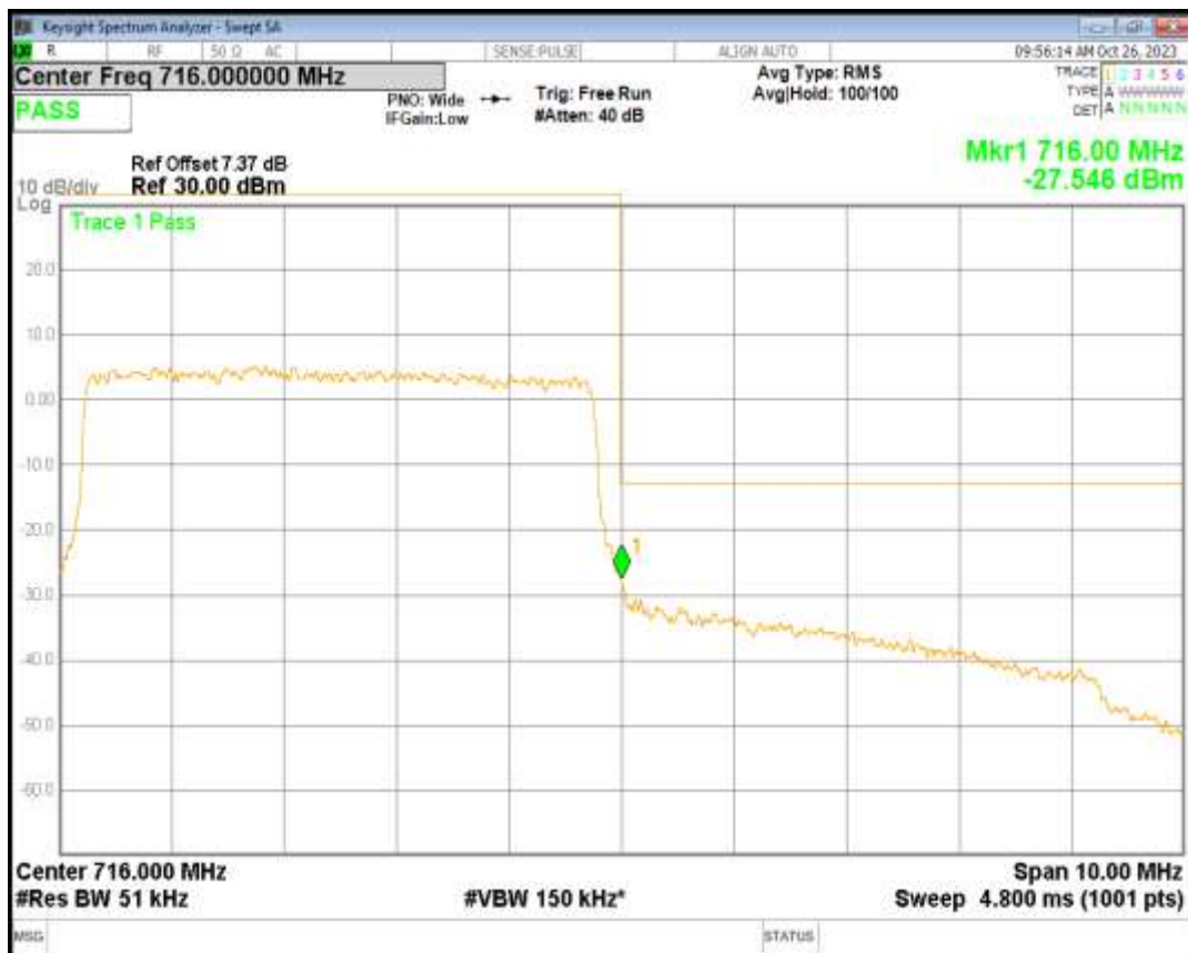
Band2 16QAM BW=1.4MHz Channel=18607 RB Size=6 Position=#0
