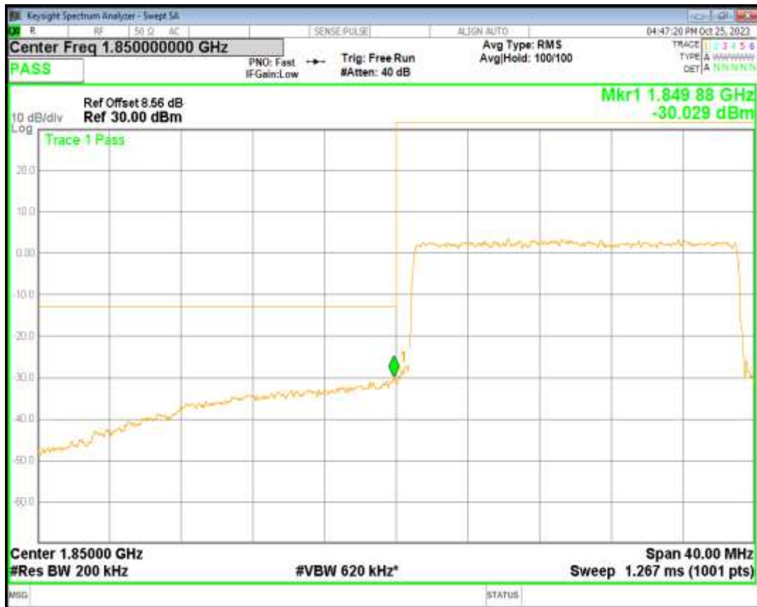
Band2 16QAM BW=20MHz Channel=19100 RB Size=100 Position=#0
