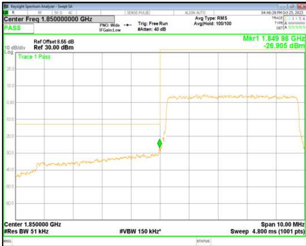
Band2 QPSK BW=5MHz Channel=19175 RB Size=25 Position=#0
