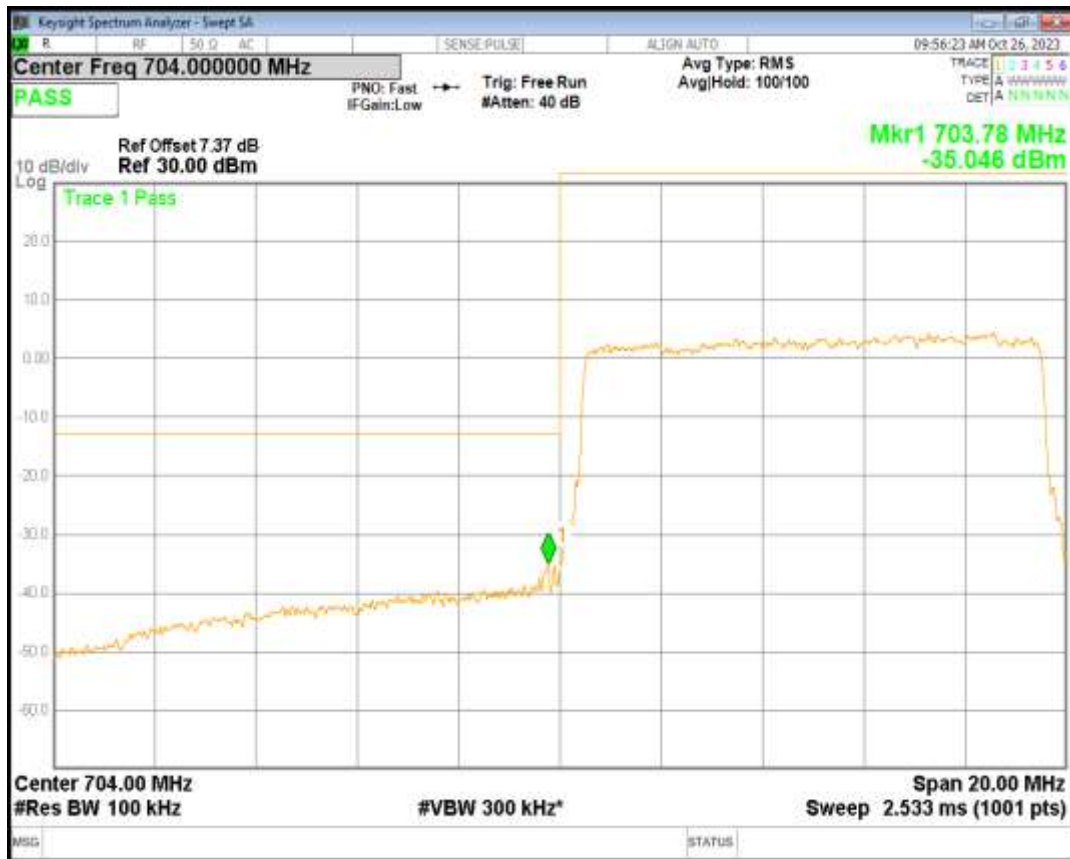
Band17 16QAM BW=10MHz Channel=23800 RB Size=50 Position=#0
