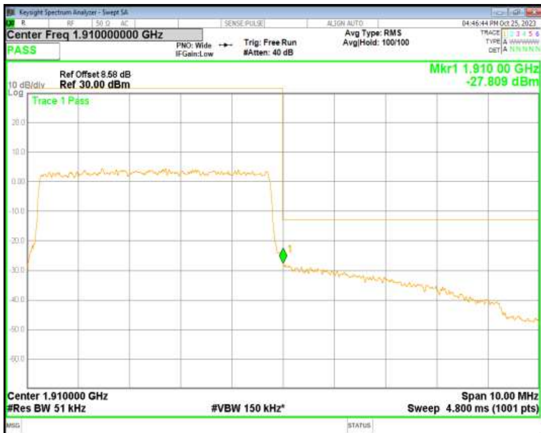
Band25 16QAM BW=1.4MHz Channel=26047 RB Size=6 Position=#0
