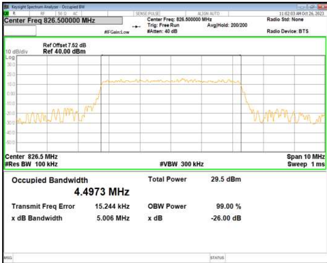
Band26(824-849) 16QAM BW=5MHz Channel=26915 RB Size=25 Position=#0
