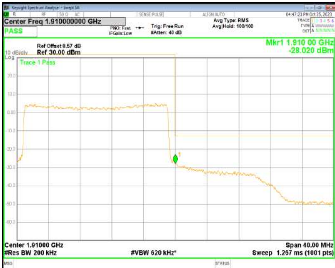
Band2 QPSK BW=3MHz Channel=18615 RB Size=15 Position=#0
