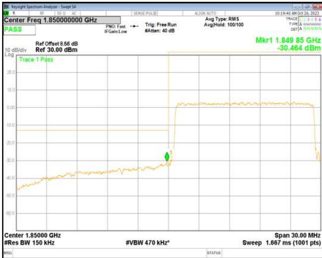
Band25 16QAM BW=15MHz Channel=26615 RB Size=75 Position=#0
