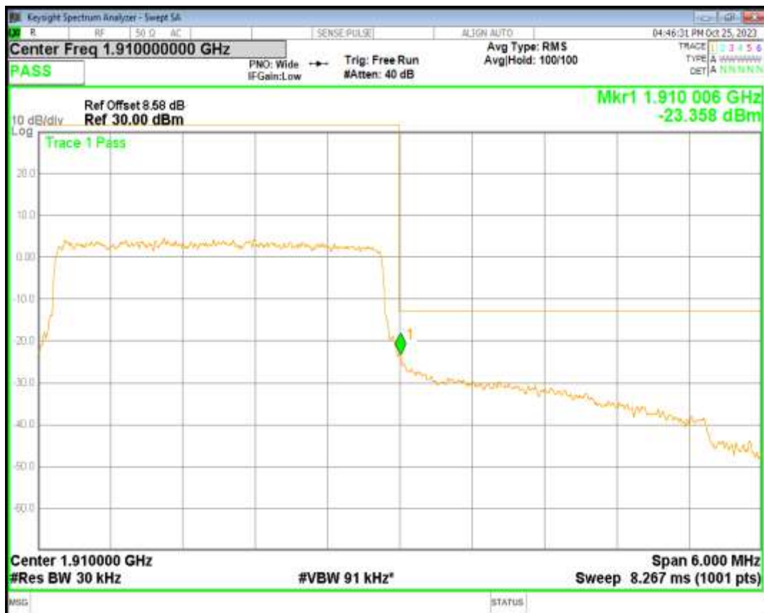
Band2 QPSK BW=5MHz Channel=18625 RB Size=25 Position=#0
