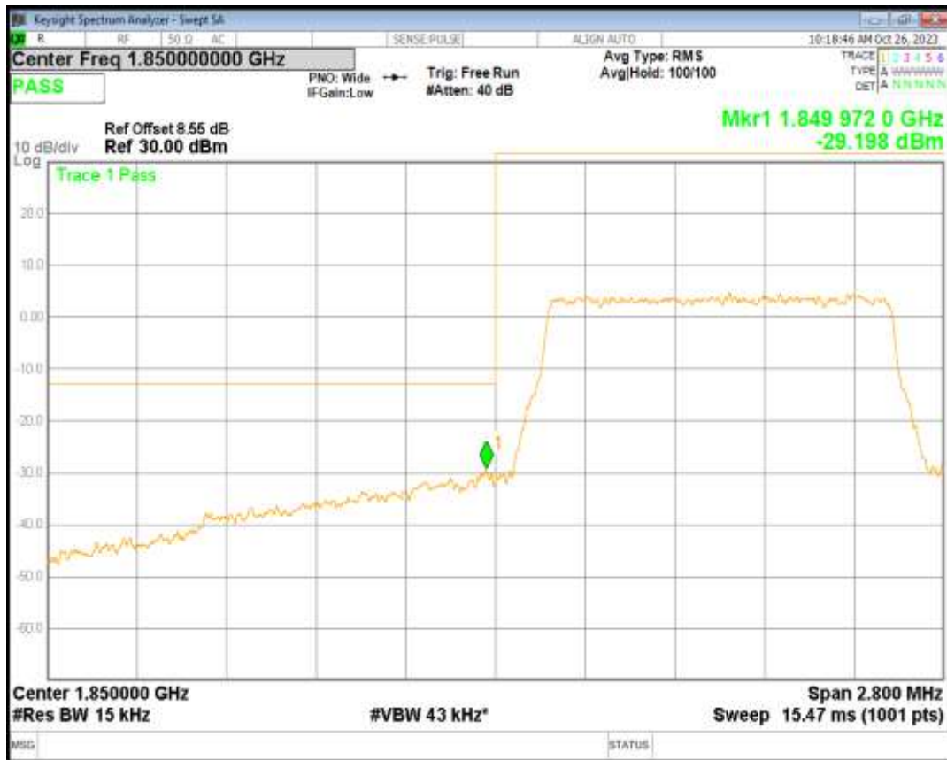
Band25 16QAM BW=1.4MHz Channel=26683 RB Size=6 Position=#0
