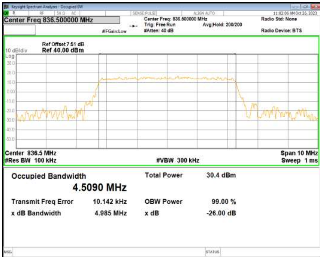
Band26(824-849) QPSK BW=5MHz Channel=27015 RB Size=25 Position=#0
