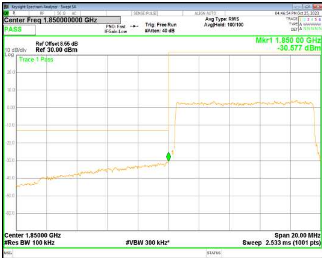
Band2 16QAM BW=10MHz Channel=19150 RB Size=50 Position=#0
