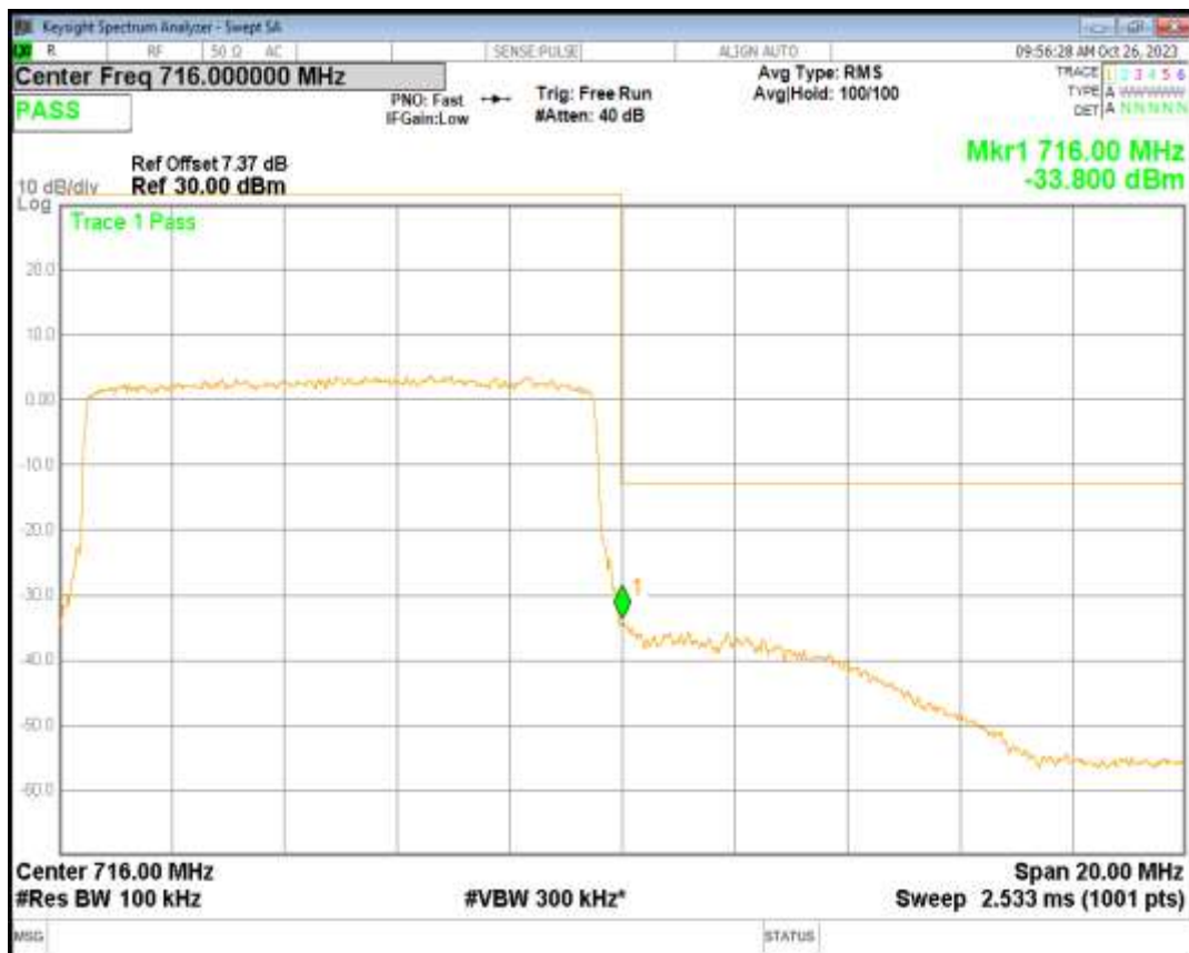
Band17 16QAM BW=5MHz Channel=23755 RB Size=25 Position=#0
