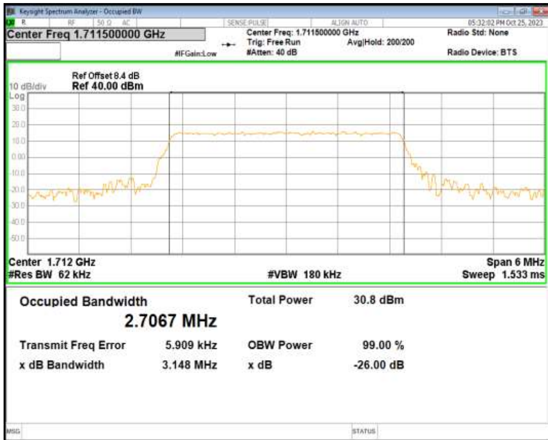
Band4 QPSK BW=3MHz Channel=20175 RB Size=15 Position=#0
