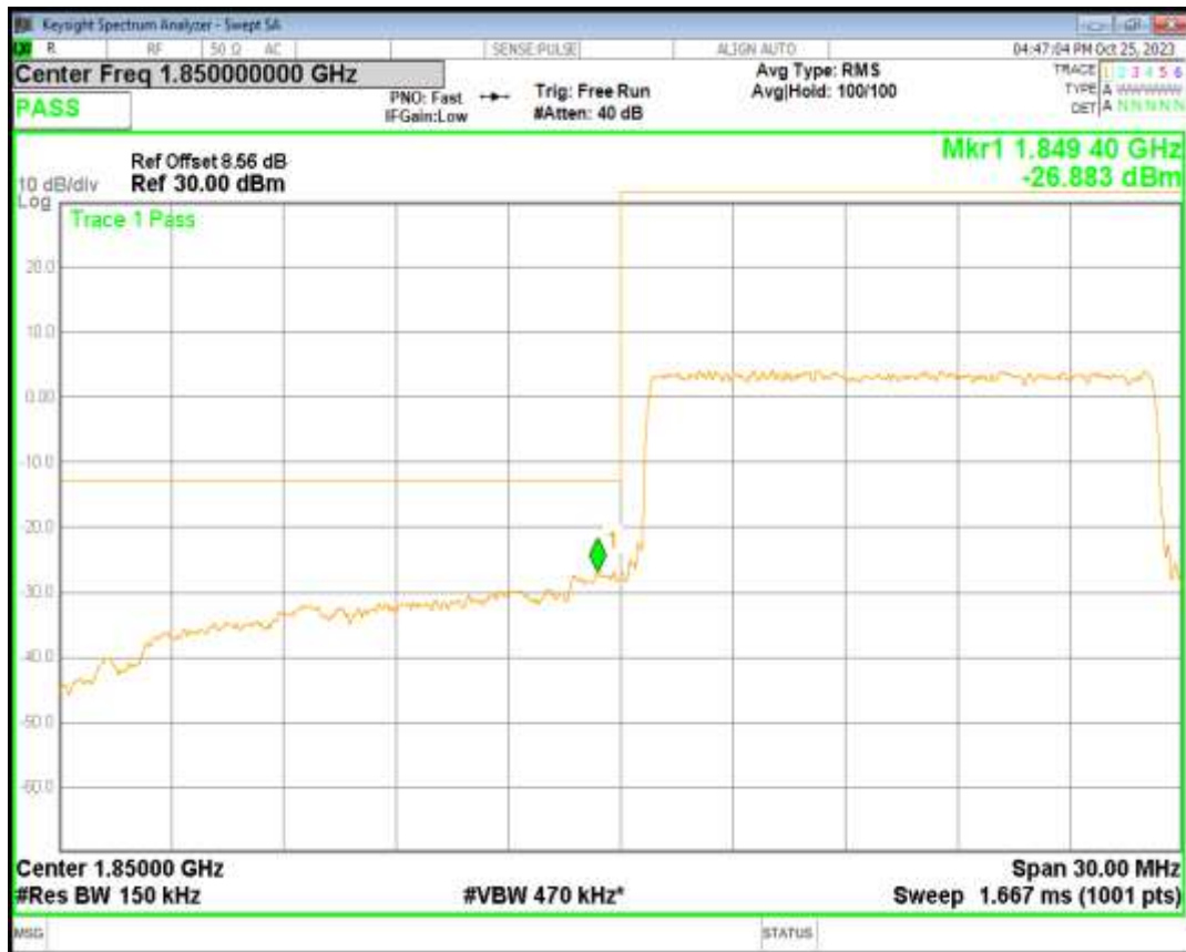
Band2 QPSK BW=15MHz Channel=19125 RB Size=75 Position=#0
