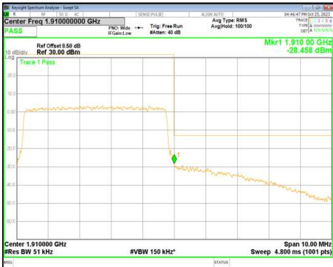
Band2 QPSK BW=1.4MHz Channel=18607 RB Size=6 Position=#0
