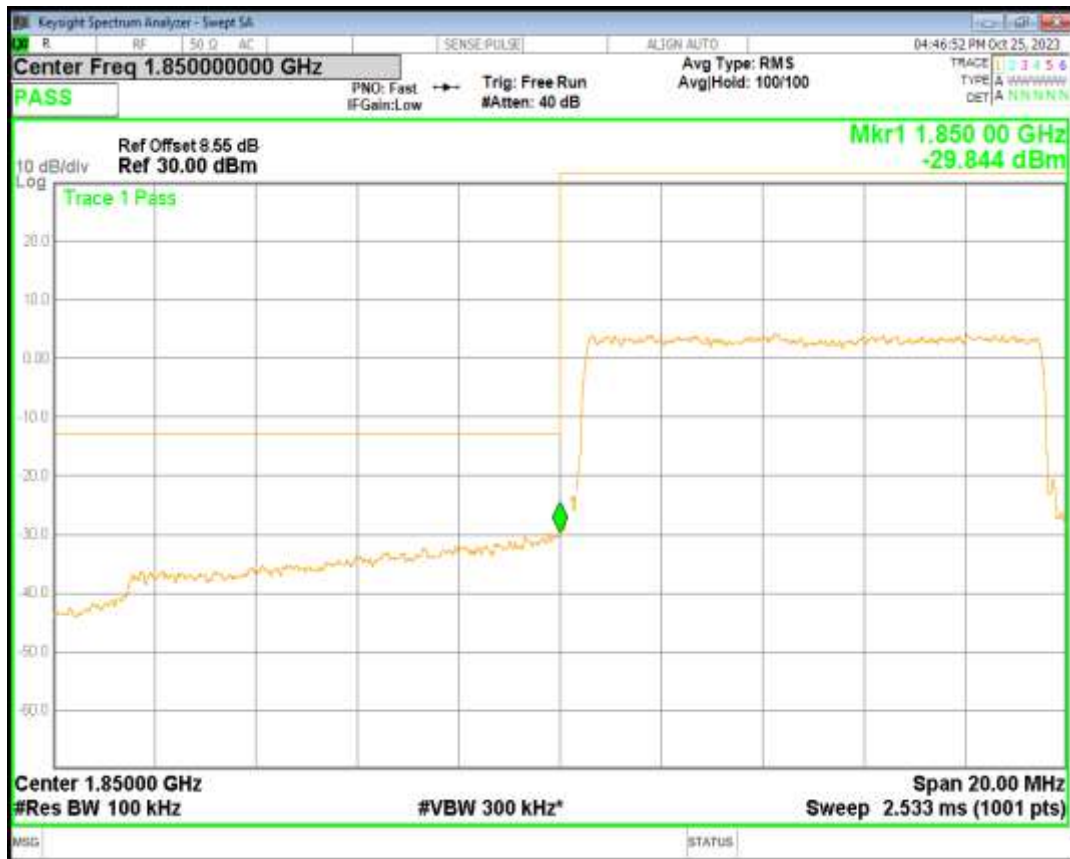
Band2 QPSK BW=10MHz Channel=19150 RB Size=50 Position=#0
