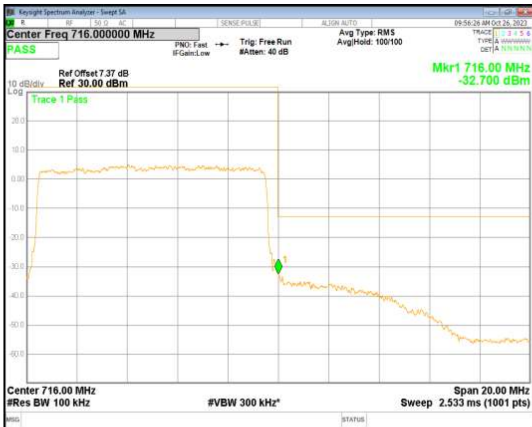
Band17 QPSK BW=5MHz Channel=23755 RB Size=25 Position=#0
