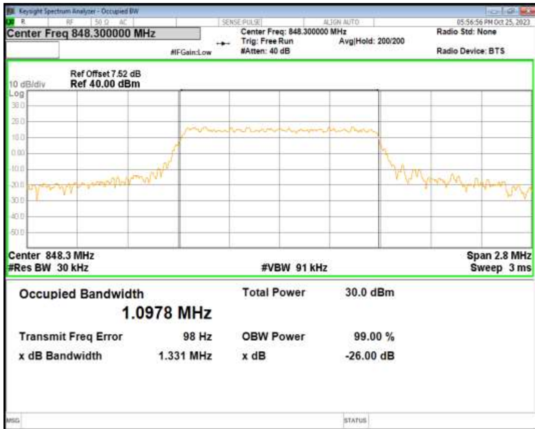
Band5 16QAM BW=10MHz Channel=20450 RB Size=50 Position=#0
