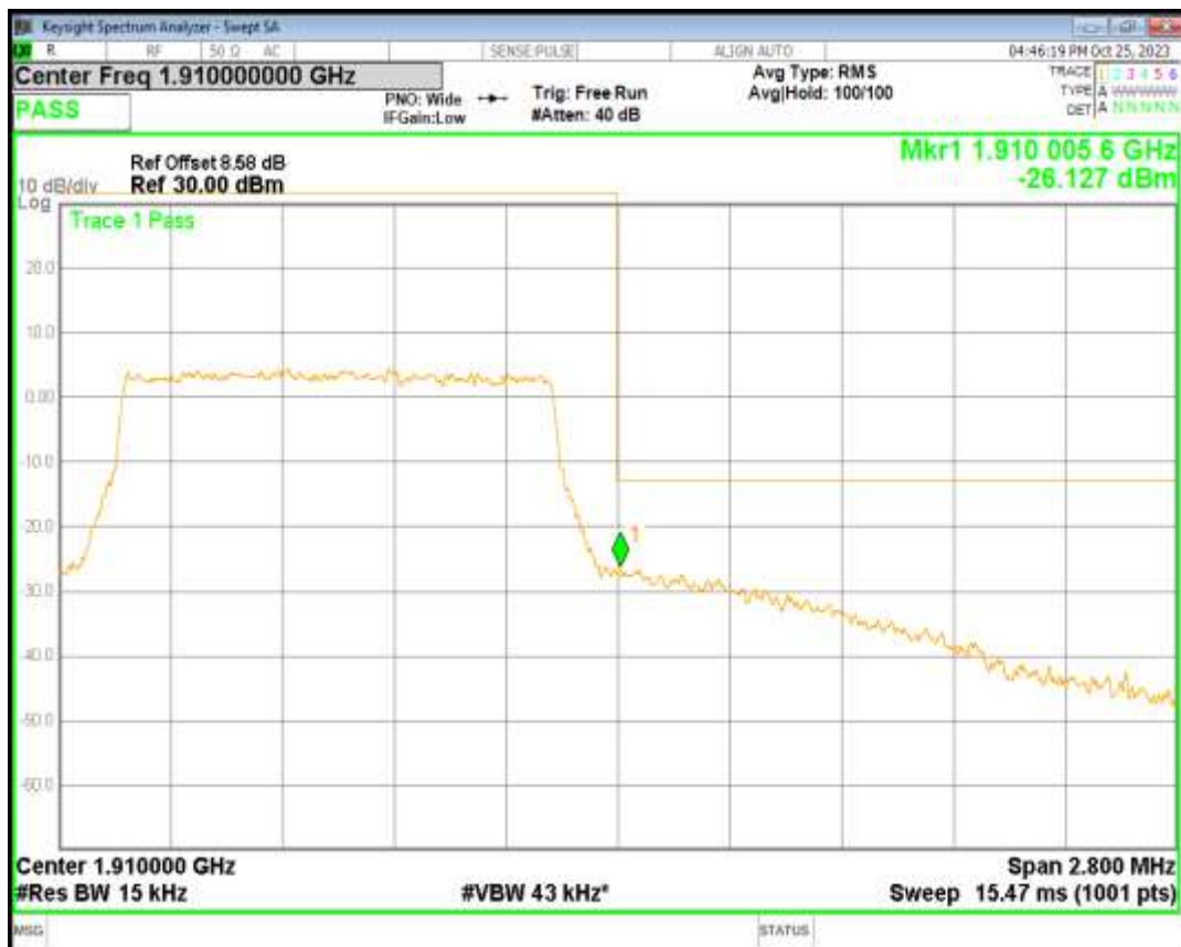
Band2 16QAM BW=10MHz Channel=18650 RB Size=50 Position=#0
