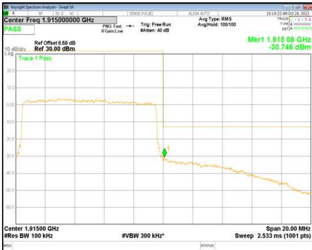
Band25 16QAM BW=15MHz Channel=26115 RB Size=75 Position=#0
