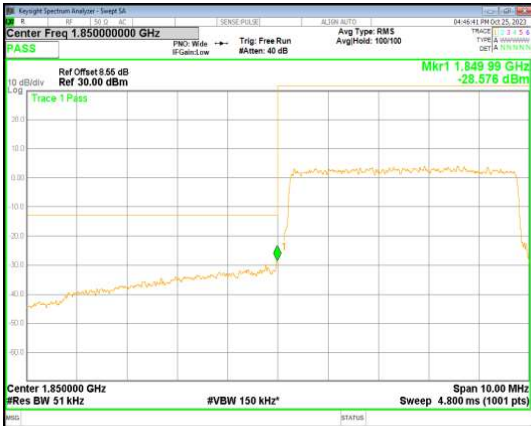
Band2 16QAM BW=5MHz Channel=19175 RB Size=25 Position=#0
