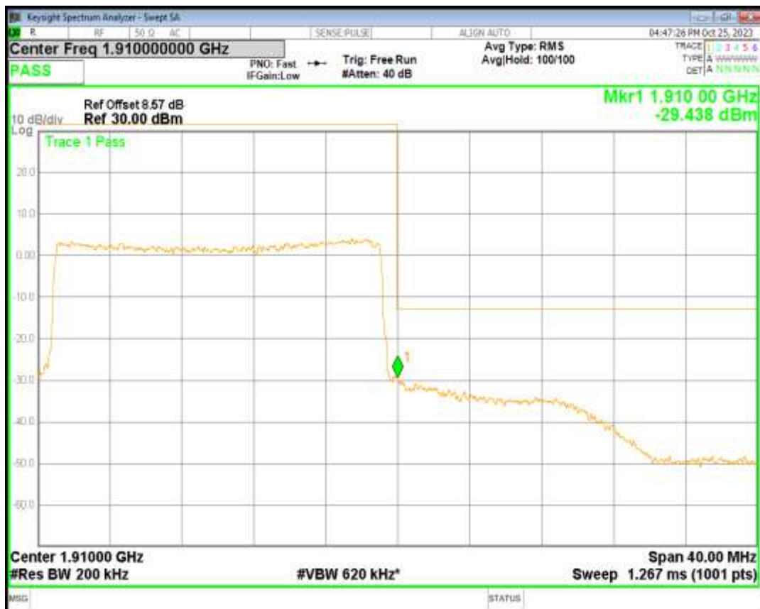
Band2 16QAM BW=3MHz Channel=18615 RB Size=15 Position=#0
