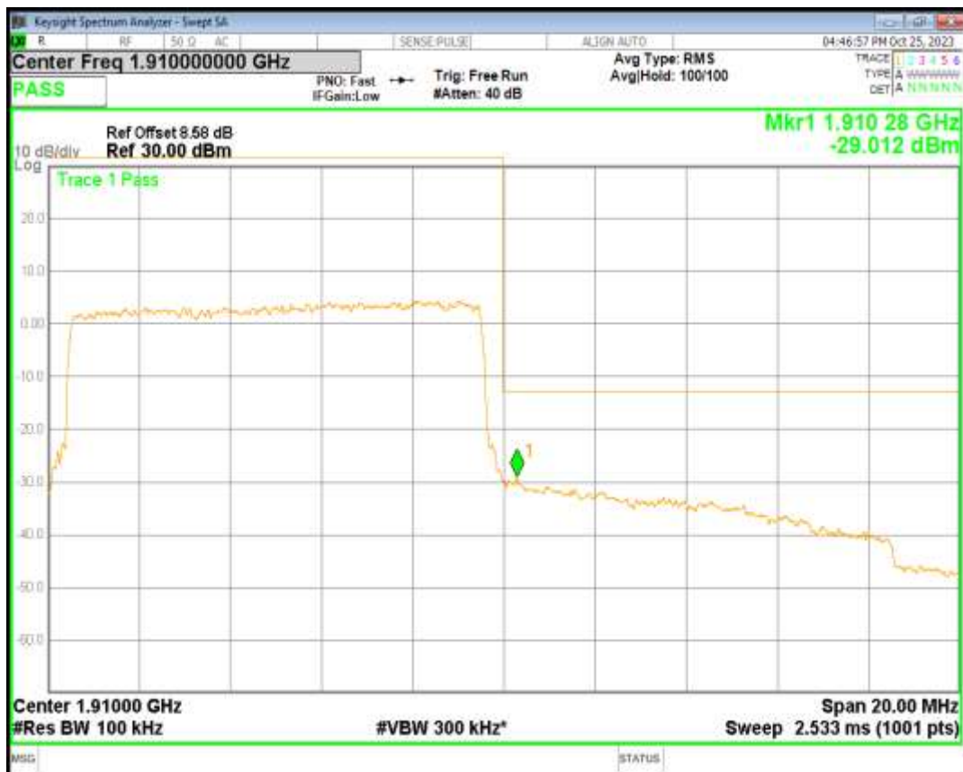
Band2 QPSK BW=15MHz Channel=18675 RB Size=75 Position=#0
