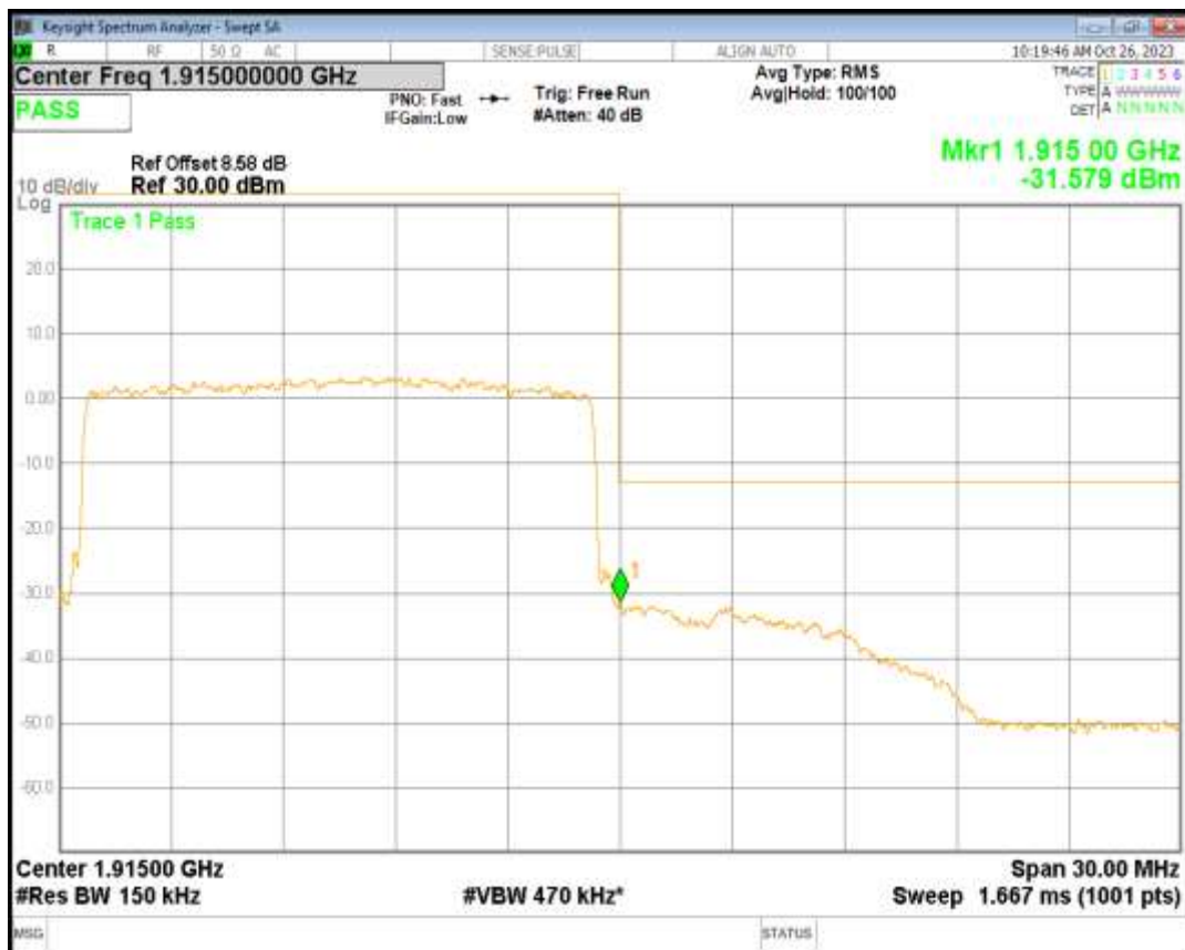
Band25 16QAM BW=20MHz Channel=26140 RB Size=100 Position=#0
