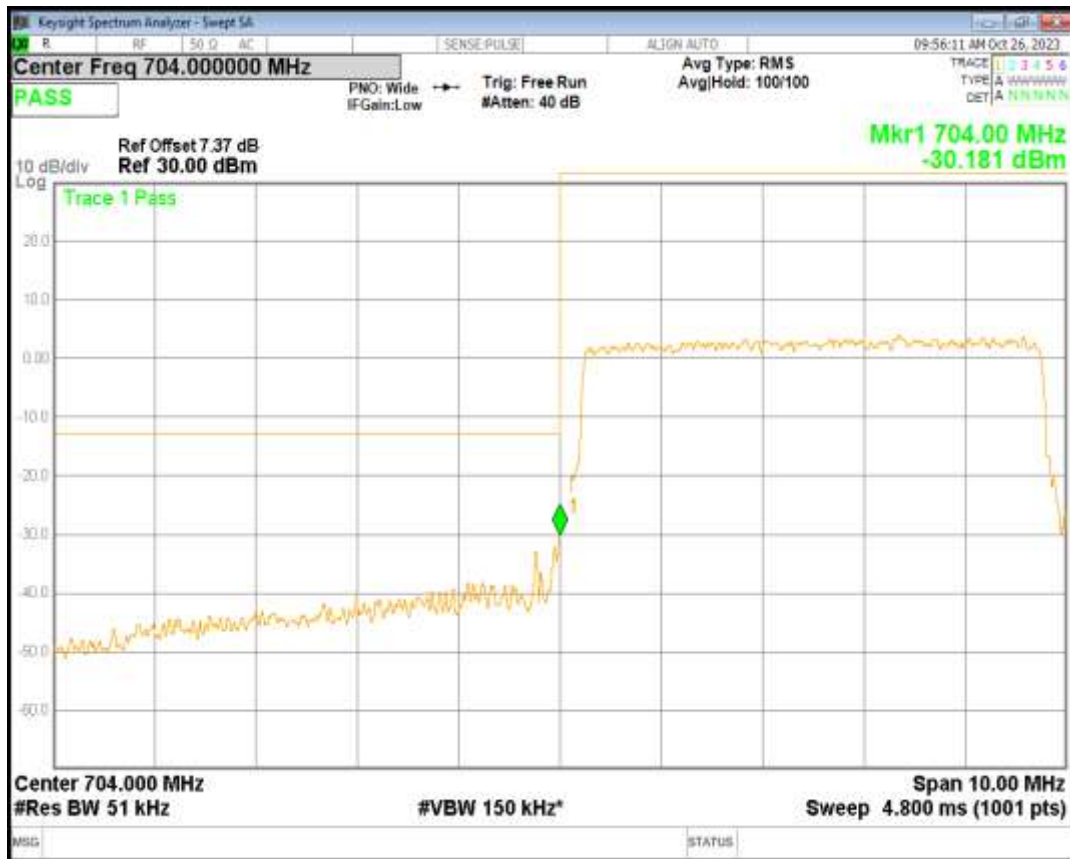
Band17 16QAM BW=5MHz Channel=23825 RB Size=25 Position=#0
