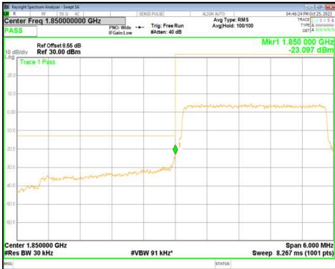
Band2 QPSK BW=3MHz Channel=19185 RB Size=15 Position=#0
