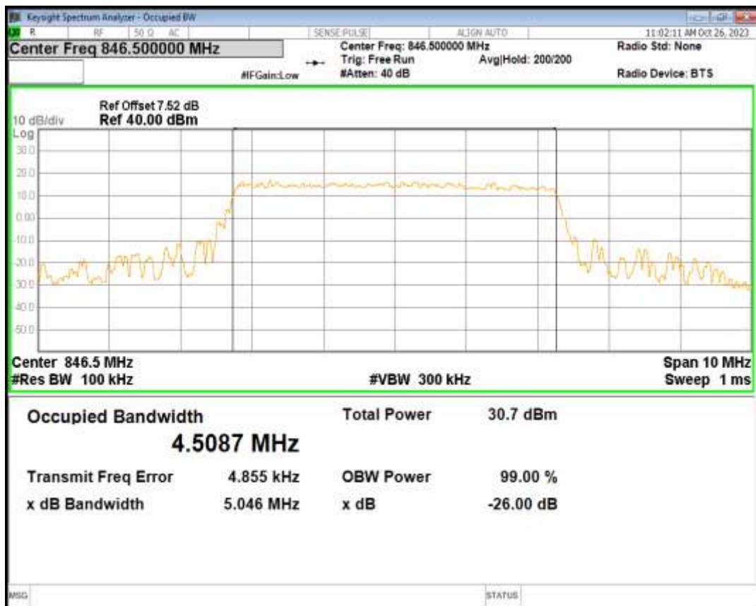
Band4 16QAM BW=1.4MHz Channel=19957 RB Size=6 Position=#0
