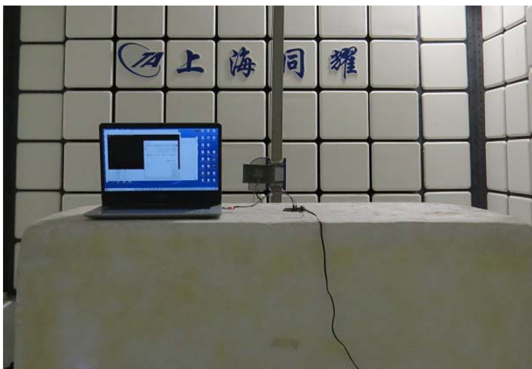
Picture 1 Radiated Emission Test Setup
