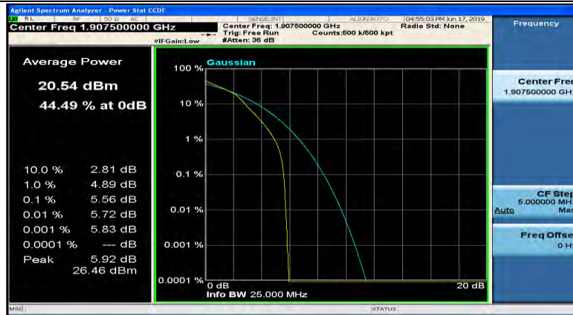
(Channel Bandwidth: 5 MHz)_HCH_16QAM_25RB#0
