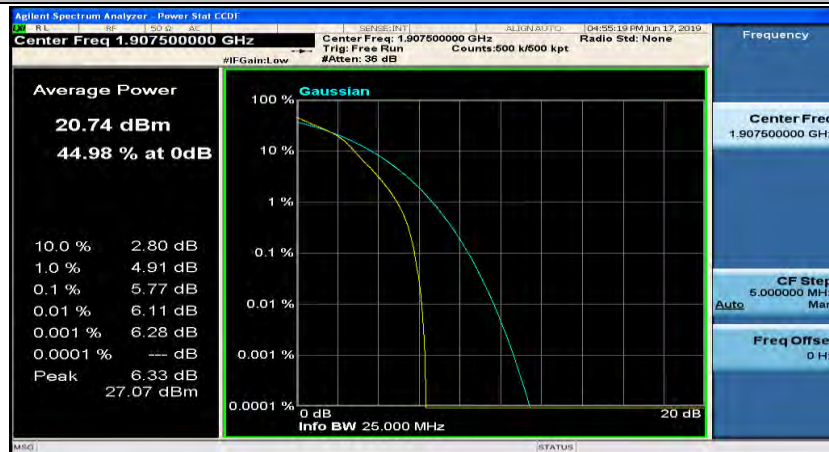
(Channel Bandwidth: 5 MHz)_HCH_16QAM_25RB#0
