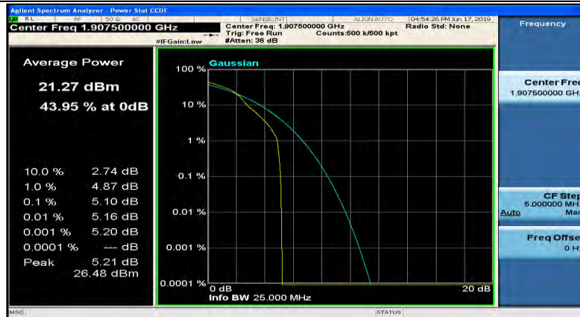
(Channel Bandwidth: 5 MHz)_HCH_16QAM_12RB#0
