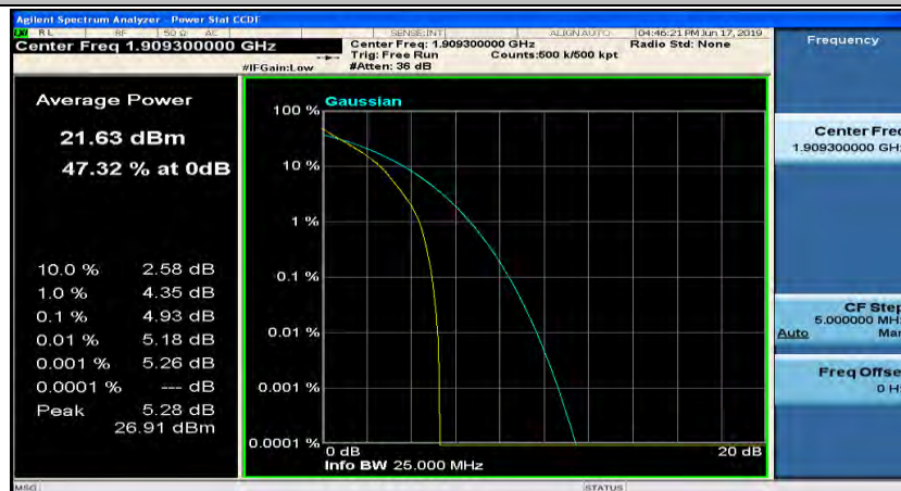
(Channel Bandwidth: 1.4 MHz)_HCH_QPSK_6RB#0
