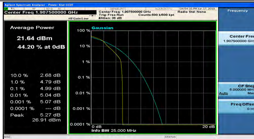
(Channel Bandwidth: 5 MHz)_HCH_16QAM_1RB#12
