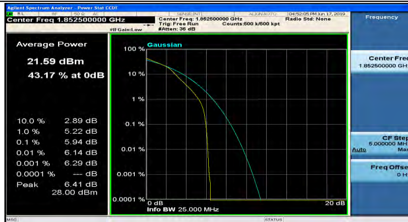
(Channel Bandwidth: 5 MHz)_LCH_16QAM_25RB#0
