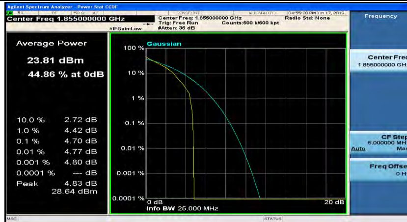
Channel Bandwidth: 10 MHz_LCH_QPSK_1RB#24
