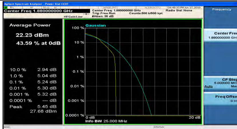
(Channel Bandwidth: 3 MHz)_MCH_16QAM_8RB#0
