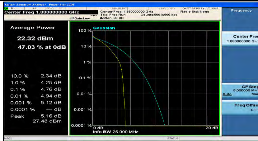
Channel Bandwidth: 10 MHz_MCH_QPSK_25RB#12
