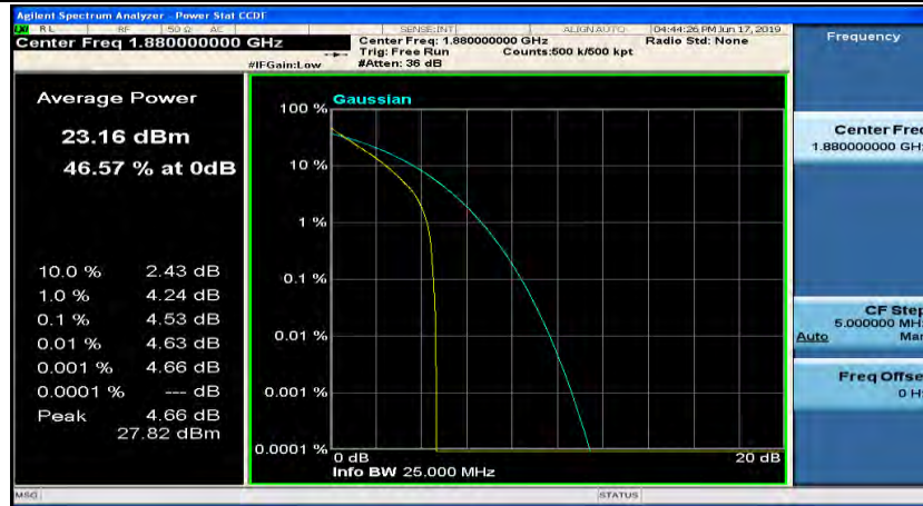
(Channel Bandwidth: 1.4 MHz)_MCH_QPSK_6RB#0
