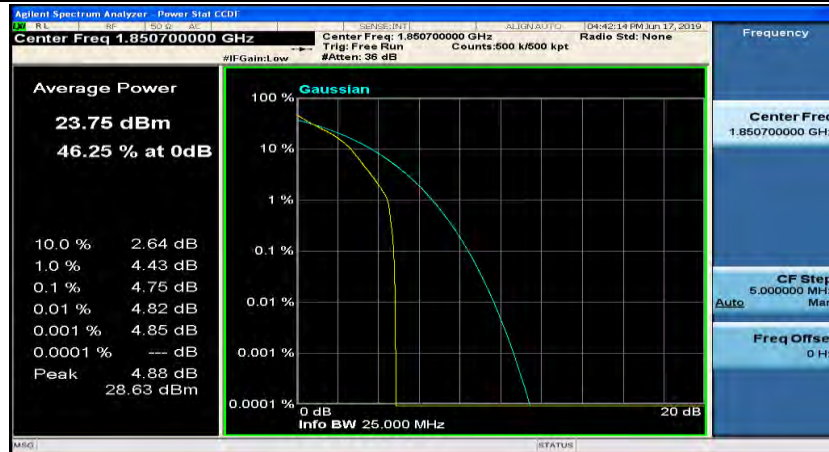
(Channel Bandwidth: 1.4 MHz)_LCH_QPSK_1RB#3
