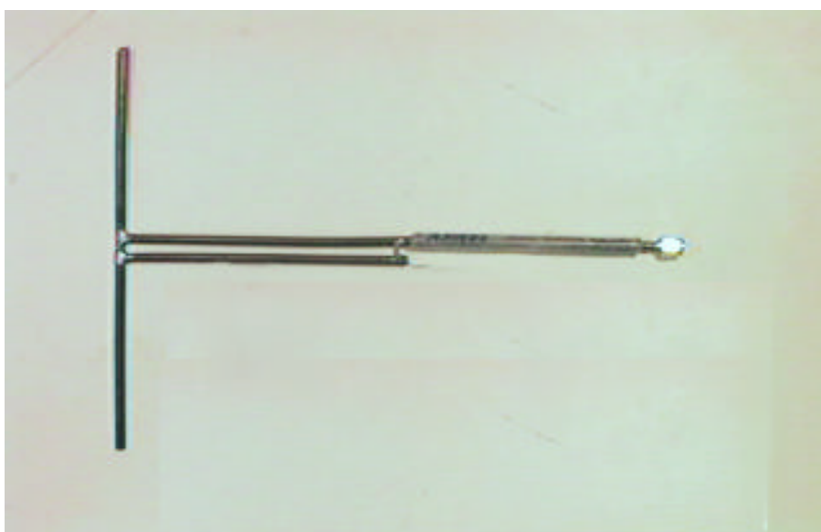
Reference Dipole Antenna Used for ERP Measurement
