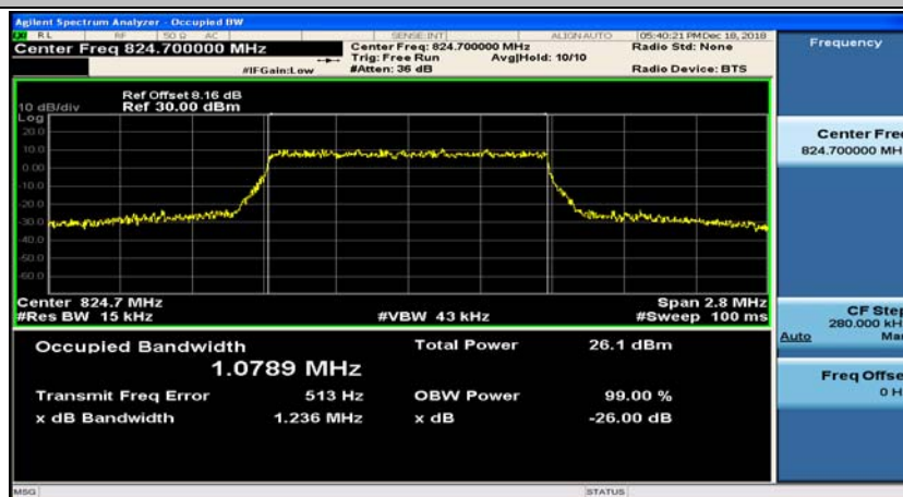
(Channel Bandwidth: 1.4 MHz)_LCH_16QAM_6RB#0
