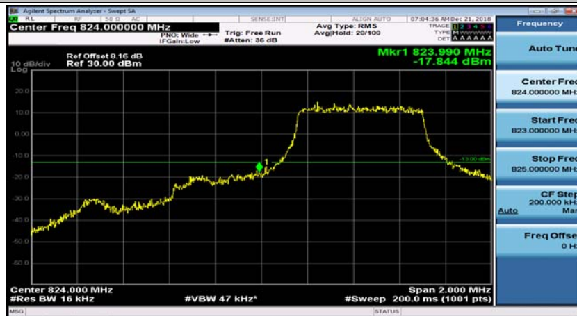
(Channel Bandwidth: 1.4 MHz)_LCH_QPSK_3RB#2
