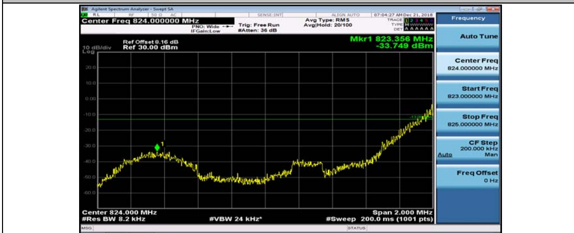
(Channel Bandwidth: 1.4 MHz)_LCH_16QAM_3RB#0
