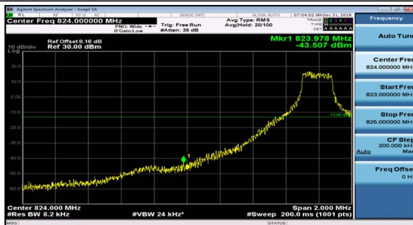
(Channel Bandwidth: 1.4 MHz)_LCH_QPSK_1RB#5
