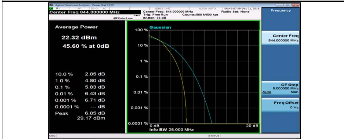
Channel Bandwidth: 10 MHz_HCH_16QAM_50RB#0
