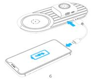
To charge a mobile device with FLIbank, pull the charging cable out by its tab and plug it in.
