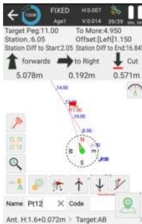
Choose a line to stake, set Offset, Cross-Section Slope and Stakeout by Pile-to-Pile Coordinate parameters.
