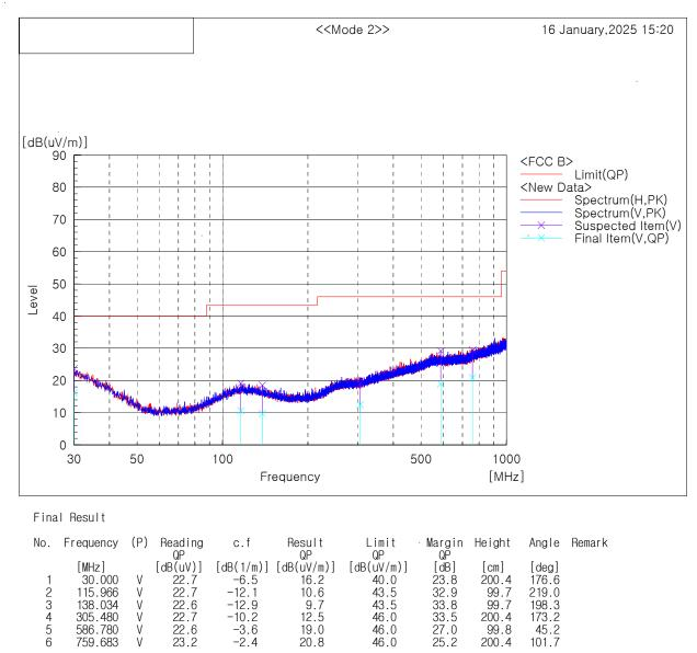
Note1) Receiving antenna polarization : Horizontal, Vertical Test Distance : 3 m, Antenna Height : 1 to 4 meters Result (QP) = Reading (QP) + c.f (Antenna Factor + Cable Loss - Amp. Gain) Margin (QP) = Limit – Level (QP) QP = Quasi-Peak, c.f = Correction Factor
