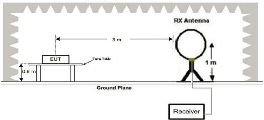
2. Radiated Emission Test-Up Frequency 30MHz~1GHz
