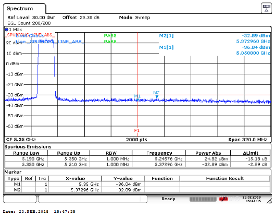
Figure 9 Spurious Emissions (Upper Band Edge) – 256QAM (5240.0 MHz) (20MHz Channel BW)
