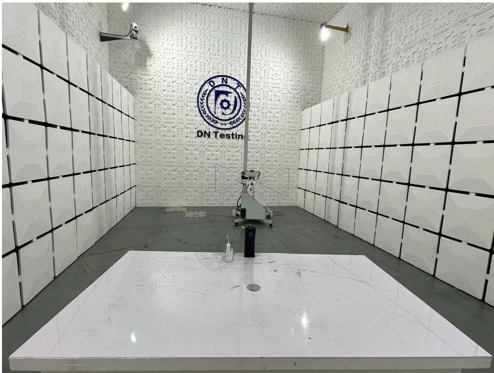
Radiated Emission Test View|(Below 1G)
