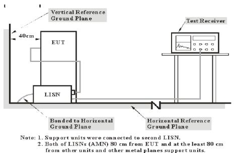
The setup of EUT is according with per ANSI C63.10-2013 measurement procedure. The specification used was with the FCC Part 15.207,RSS-Gen limits.
