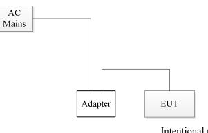
Intentional radiator circuitry of EUT 120 cm above Ground Plane
