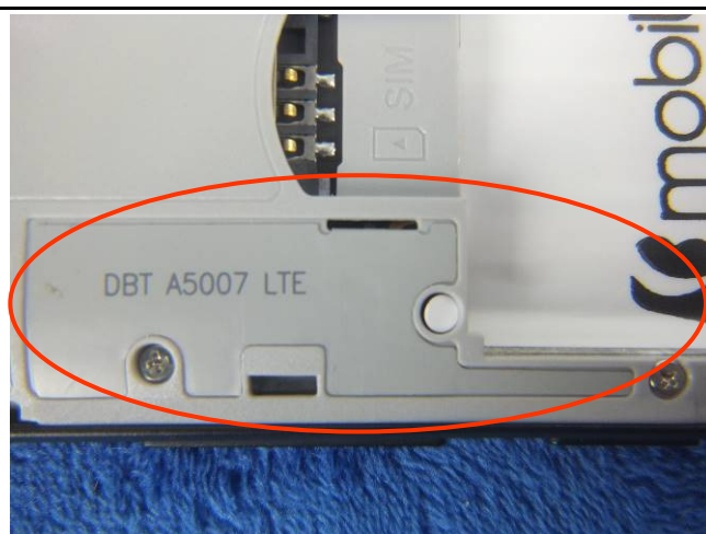
LTE- Antenna View
