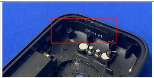
The antenna is FPC antenna. The best case gain of the antenna is 1.13dBi.
