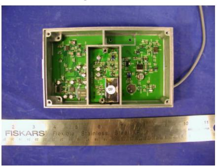
**EUT – Transmitter Solder View**
