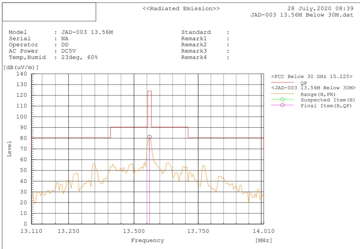
Antenna Polarity & Test Distance: Loop Antenna 0 degree At 3m
