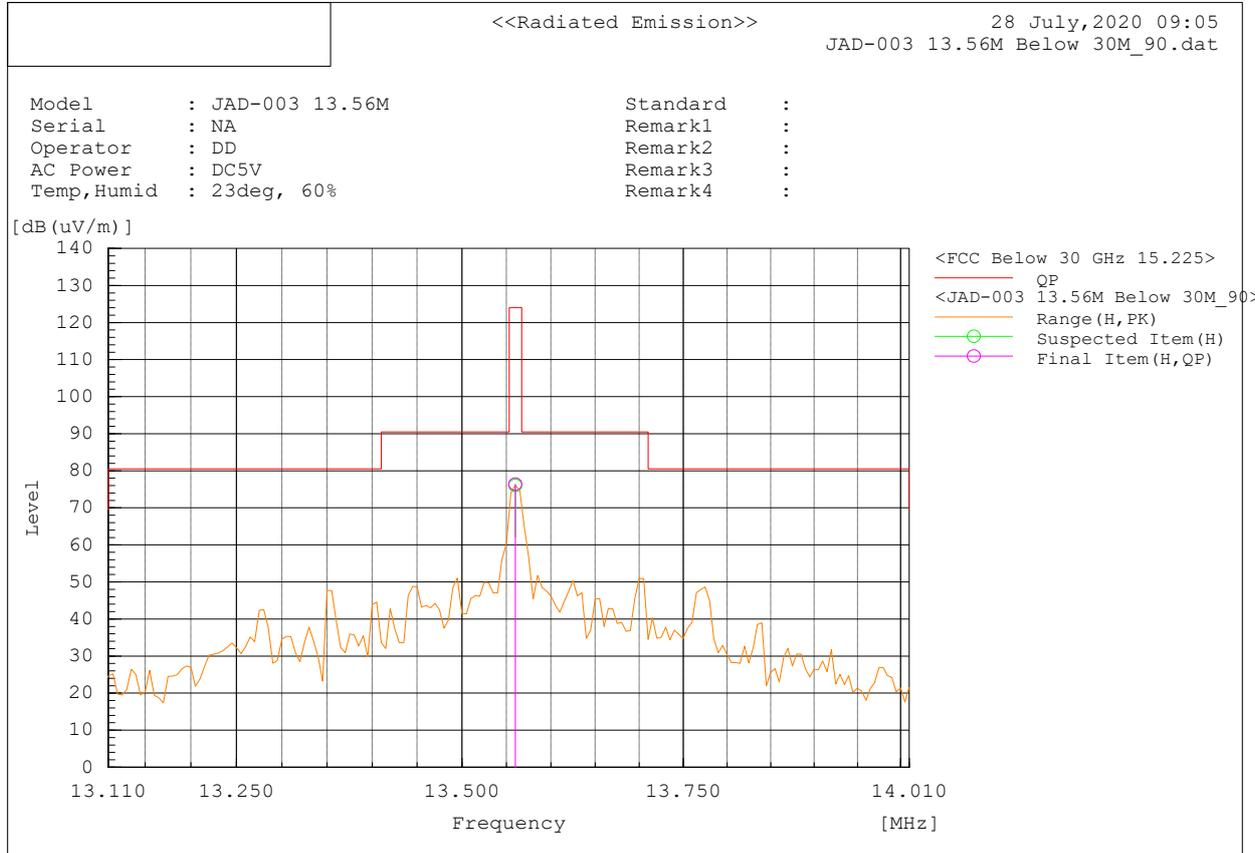
**Antenna Polarity & Test Distance: Loop Antenna 90 degree At 3m**
