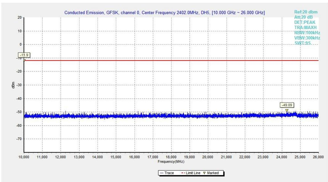
Fig.23. Conducted spurious emission: GFSK, Channel 0, 10GHz - 26GHz
