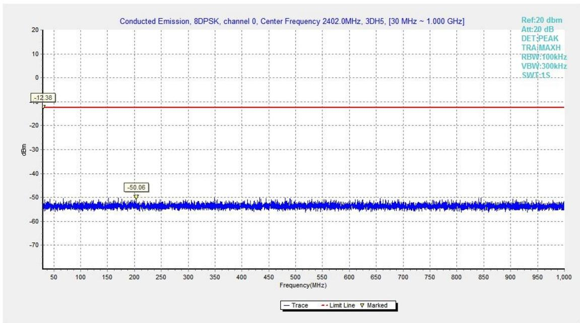
Fig.50. Conducted spurious emission: 8DPSK, Channel 0, 30MHz - 1GHz
