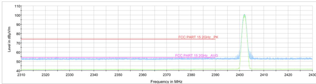
Fig.13. Frequency Band Edges: GFSK, Channel 0, Hopping Off, 2.38 GHz – 2.45GHz
