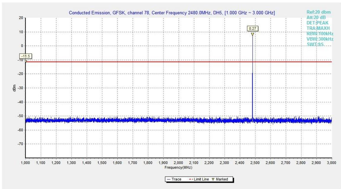
Fig.31. Conducted spurious emission: GFSK, Channel 78, 1GHz - 3GHz
