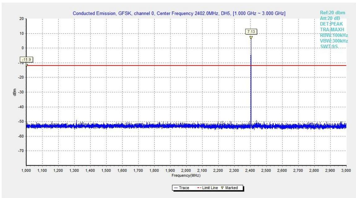
Fig.21. Conducted spurious emission: GFSK, Channel 0, 1GHz - 3GHz
