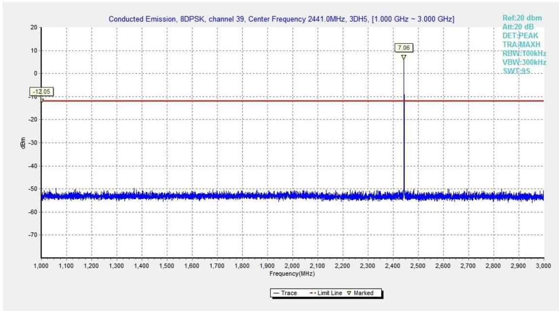
Fig.56. Conducted spurious emission: 8DPSK, Channel 39, 1GHz - 3GHz
