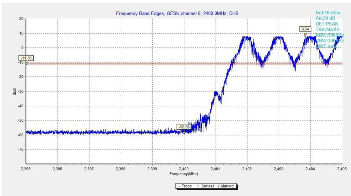
Fig.2. Frequency Band Edges: GFSK, Channel 0, Hopping On
