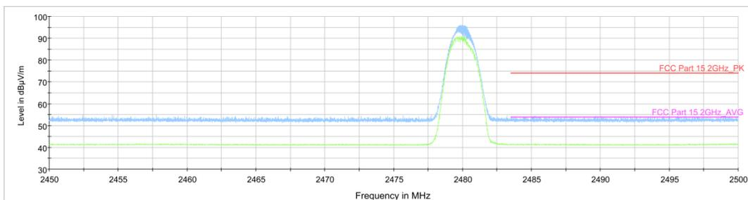
**Fig.18. Frequency Band Edges: 8DPSK, Channel 78, 2.38 GHz - 2.45GHz**
