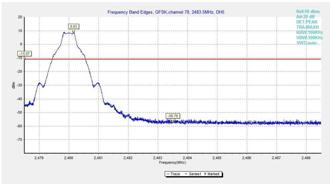
Fig.3. Frequency Band Edges: GFSK, Channel 78, Hopping Off
