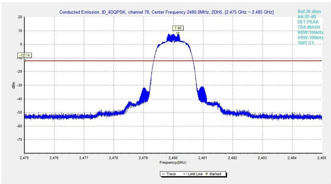
Fig.44. Conducted spurious emission:  $\pi/4$  DQPSK, Channel 78, 2480MHz
