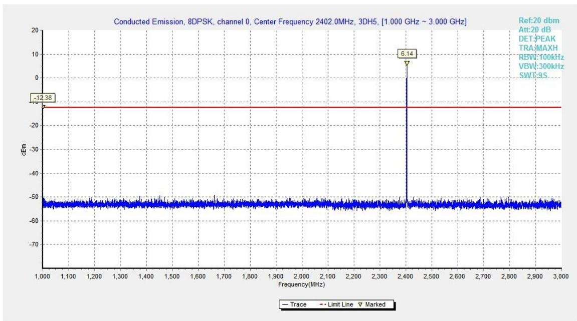
Fig.51. Conducted spurious emission: 8DPSK, Channel 0, 1GHz - 3GHz
