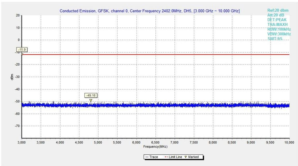
Fig.22. Conducted spurious emission: GFSK, Channel 0, 3GHz - 10GHz
