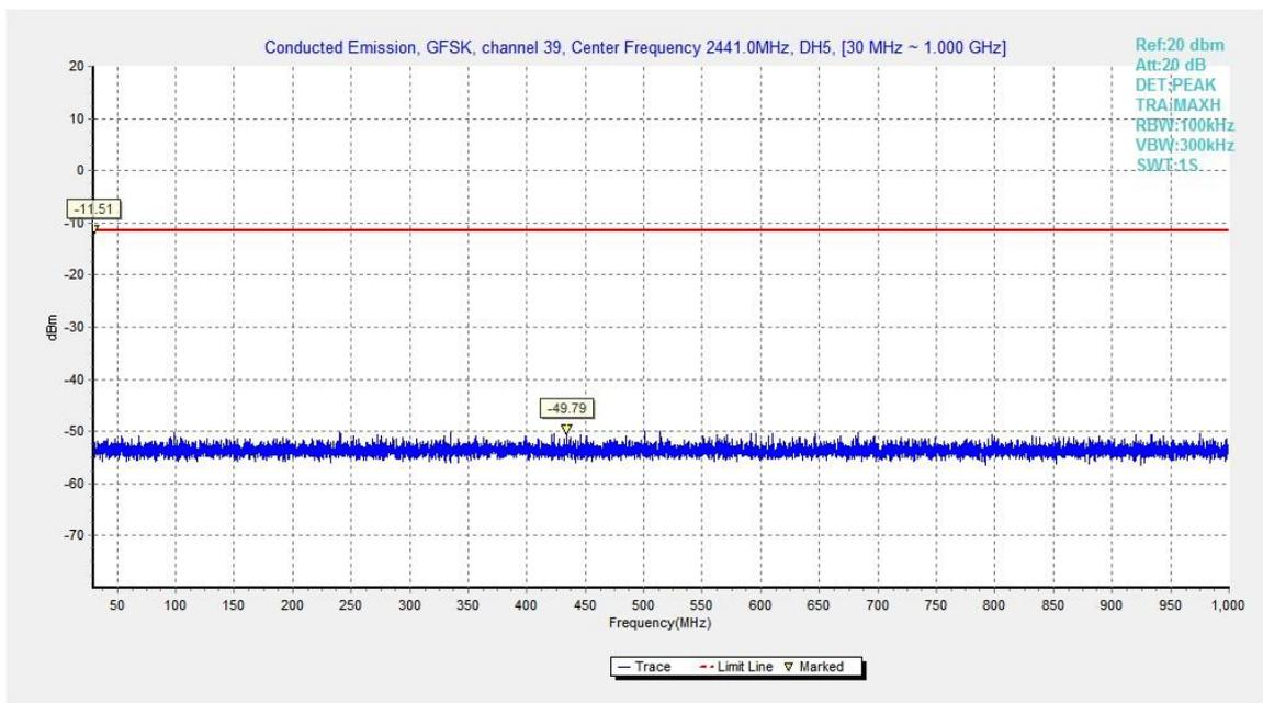
Fig.25. Conducted spurious emission: GFSK, Channel 39, 30MHz - 1GHz
