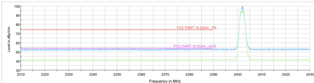
**Fig.17. Frequency Band Edges: 8DPSK, Channel 0, 2.38 GHz - 2.45GHz**
