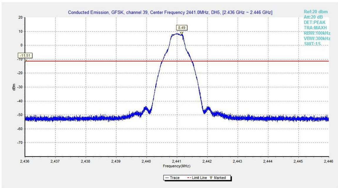
Fig.24. Conducted spurious emission: GFSK, Channel 39, 2441MHz
