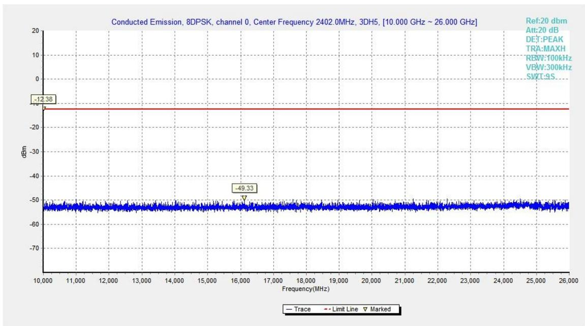
Fig.53. Conducted spurious emission: 8DPSK, Channel 0, 10GHz - 26GHz
