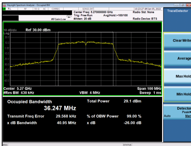
Plot 7-27. 26dB BW & 99% OBW Antenna WF8 (40MHz BW 802.11n – Ch. 54, MCS3)
