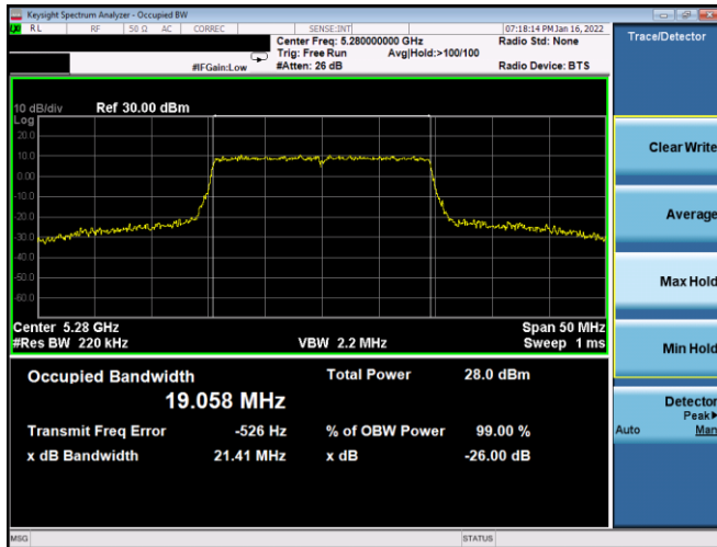
Plot 7-26. 26dB BW & 99% OBW Antenna WF8 (20MHz BW 802.11ax(SU) – Ch. 56, MCS3)
