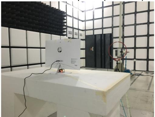
Radiated Emission Set up Photos (Below 1GHz)
