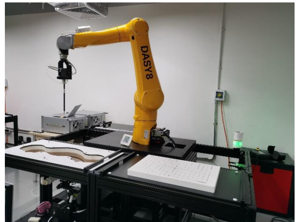
Picture D.6 Specific Absorption Rate Test Layout
