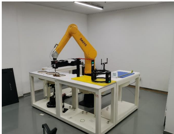
Picture D.6 Specific Absorption Rate Test Layout
