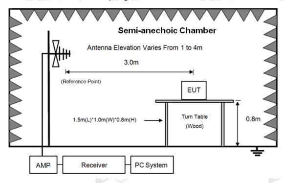
Semi-Anechoic 3m Chamber
